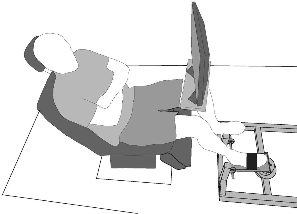
**Figure 4.** Subject was seated in a chair with the right foot strapped to a force transducer. The monitor provided force and EMG feedback to the subject.
