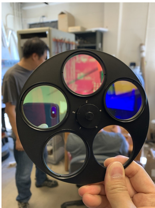
Figure 2.3: The Filter Wheel The lenses are reflecting light as well as transmitting and so the apparently green lens(denoted by slot 2) is the red filter, the apparently red lens(slot 3) is the green filter, and the apparently blue lens(slot 4) is indeed the blue filter. Slot 1 contains the Luminescence filter.
