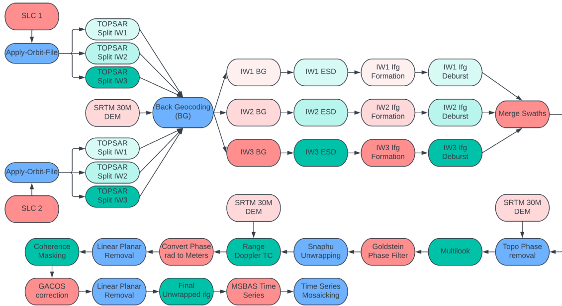
Figure 2.3.3: Workflow for creation of interferograms for time series mosaicking. Using the Sentinel1 toolbox developed by ESA.
