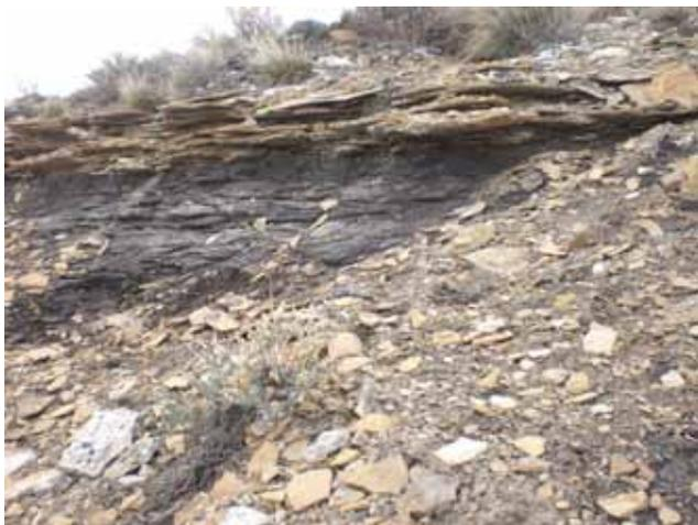
VDS at 175 feet - Underdeveloped coal bed beneath EP1 with fissile mudstone above.
