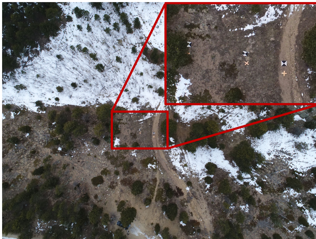
FIGURE 3 Aerial red–green–blue (RGB) photograph captured using a Da-Jiang Innovations (DJI) Phantom 4 Pro on 23 January 2020 at 120 m of altitude above ground level. The photograph depicts three ground control points (GCPs) each of two different types in the center of the image: 1-m-long spray-painted orange cotton drop cloth in an “X” pattern and 1 \times 1 \text{ m}^2 of cotton drop cloth spray-painted with black triangles. The GCPs are progressively more conspicuous under the canopy, in the shrub field, and on the dirt road. The size of the area covered by the main photograph is approximately 180 m wide \times 120 m high.
