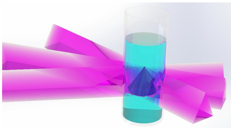
Figure 1.5. Volumetric additive manufacturing enables simultaneous 3D printing of a cone via tomographic triangular projections.
