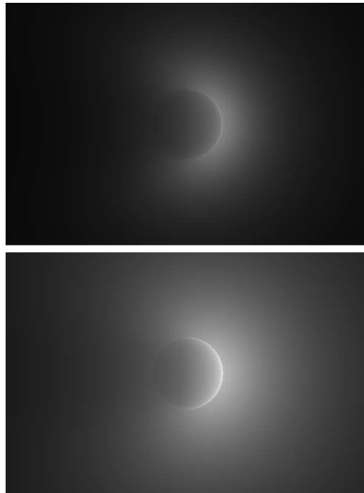
Figure 6.10: Reproduction of Figure 3.6, showing simulated coronal brightness for Chamberlain exospheres at different temperatures. As the temperature increases, the corona grows brighter and more extended but the shape is unchanged.
