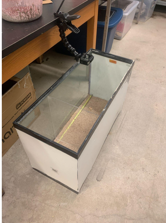
Figure 2. The experiment arena, with the glass panel and camera fixed on the tank. A tape measure was placed inside the tank to help determine the scale of the recorded video. The sides of the tank were covered with white cardboard to reduce visual distractions.
