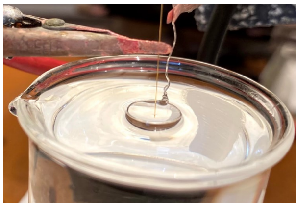
Figure 2: A close-up view of the tip-etching apparatus, showing the Au wire in an etching solution, perpendicular to the solution surface and in the center of a platinum ring.
