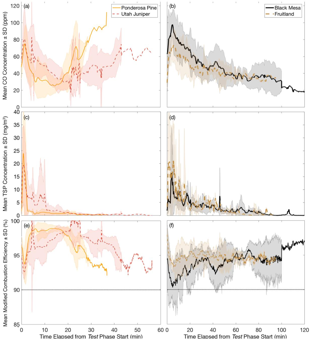
**Figure 3-5. Real-time *Test Phase* (a,b) CO and (c,d) TSP Concentrations, and (e,f) MCE. Mean Concentration is Plotted as a Solid or Dashed Line. Standard Deviation of All *Test Phases* is Plotted as Shaded Region.**
