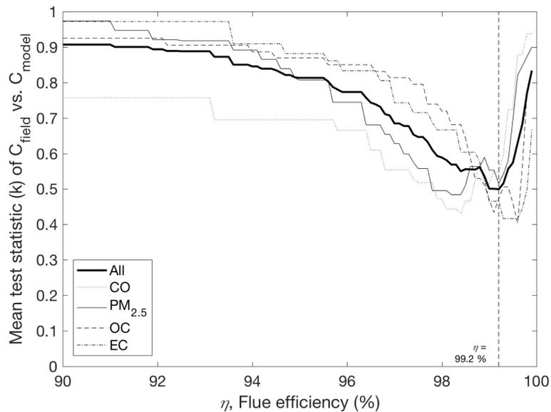
**Figure 4-2. Optimization of Flue Efficiency to Fit *Model* Steady-state Concentrations ( $C_{\text{model}}$ ) to *Field* Determined Concentrations ( $C_{\text{field}}$ ) for PM<sub>2.5</sub>, OC, EC, and CO Using Fuel Groupings.**
