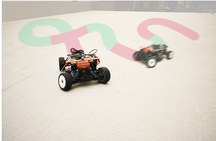
Figure 5.1: Informativeness of trajectory of parkour car where green color correspond to informative segments and red segments are non informative segments
