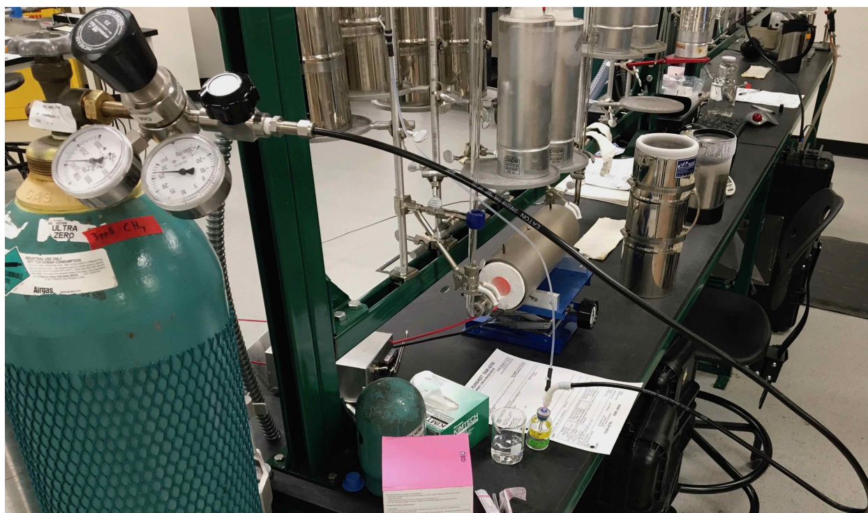
Figure D.11: Extraction of \text{CH}_4 from blue-butyl stoppered serum vial and introduction onto INSTAAR conversion line for removal of water, \text{CO}_2 , and \text{CO} , and combustion of residual gas to \text{CO}_2 .
