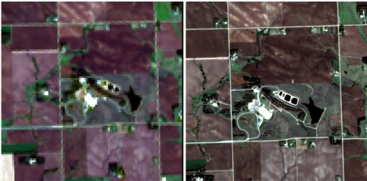
Figure 7.6. Images at the same scale with different raster resolutions, coarse (left) and fine (right). Credit: Medium Resolution Compared to High Resolution Image of USGS EROS, USGS , public domain
