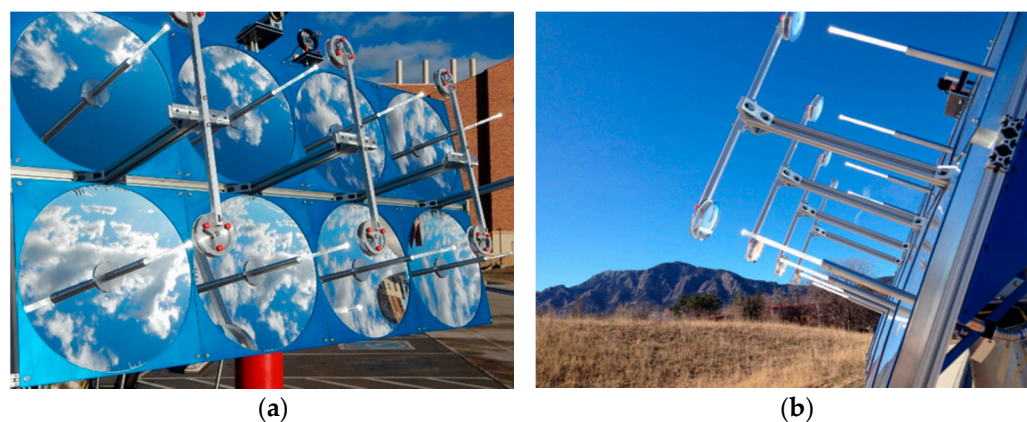
Figure 2. (a) Concentrator system on sun; (b) Detailed view of the parabolic solar concentrators actively on-sun.
