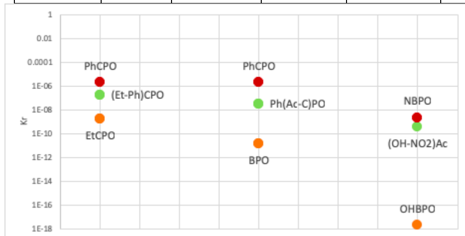
Figure S4: K_r values for asymmetric peroxides and their symmetric analogs. Asymmetric peroxides are denoted by green data points, whereas symmetric analogs are denoted by the orange and red data points.
