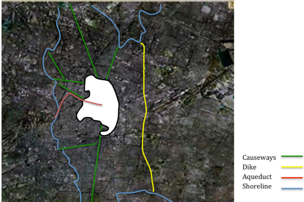
Figure 5: Hydraulic System, including the Pre-Hispanic Chapultepec aqueduct, superimposed on map of Modern Mexico City (original source).
