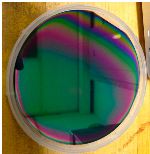
Figure 2.5: The diamond side of 0.3 \mu\text{m} thick diamond film deposited on a 500 \mu\text{m} thick Si substrate
