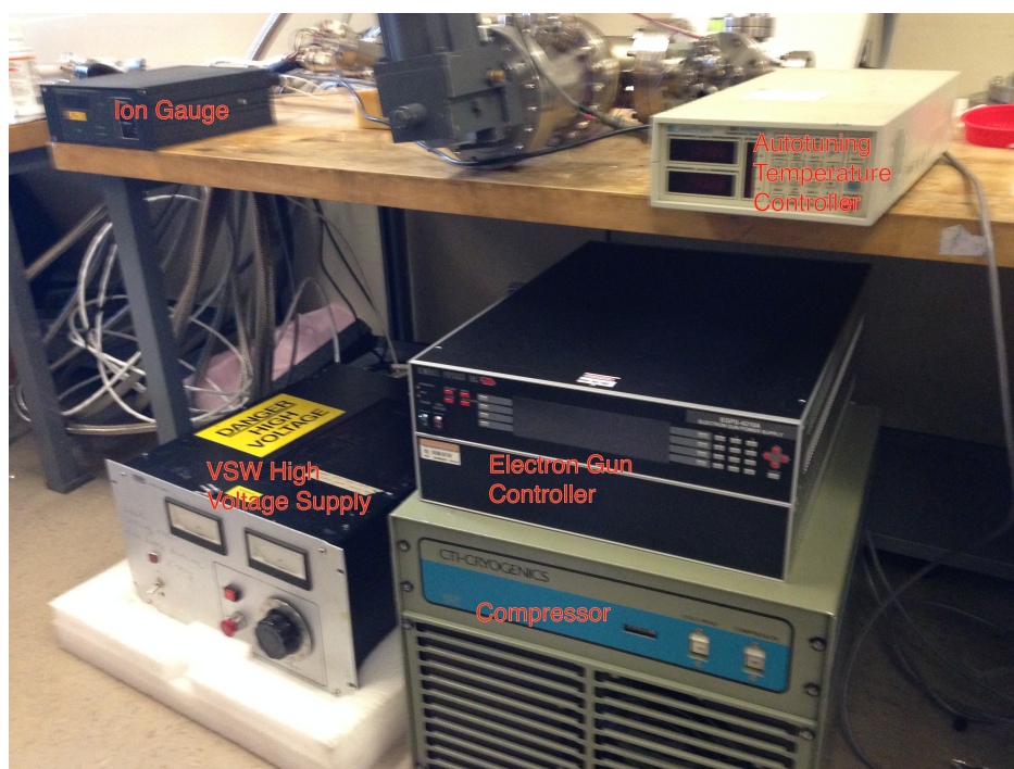
Figure 2.19: A photo of the control systems for the UV Light Source
