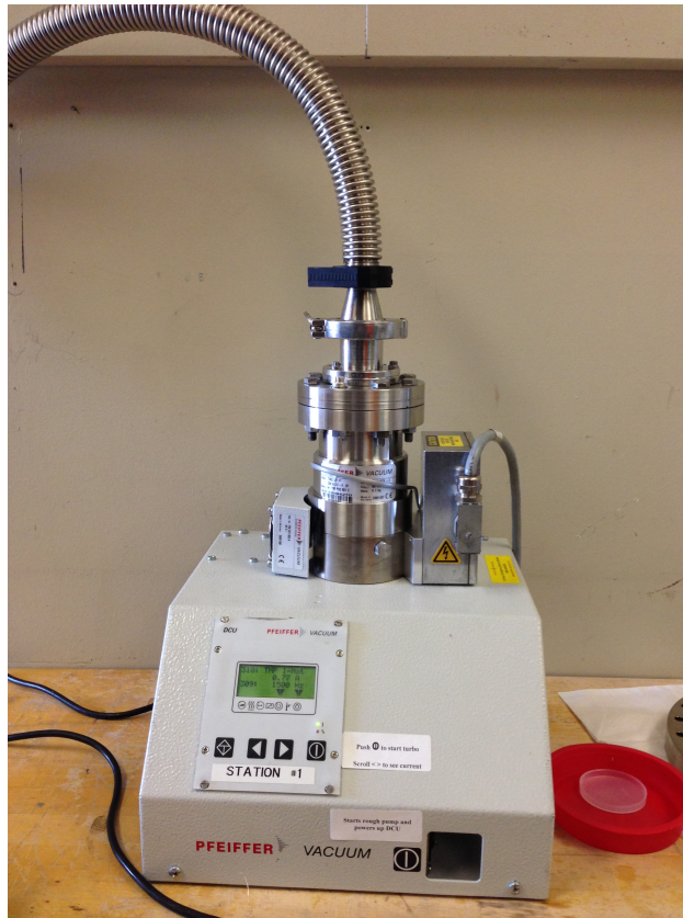
Figure 2.16: A photo of the Pfeiffer Turbo vacuum pump used for this project
