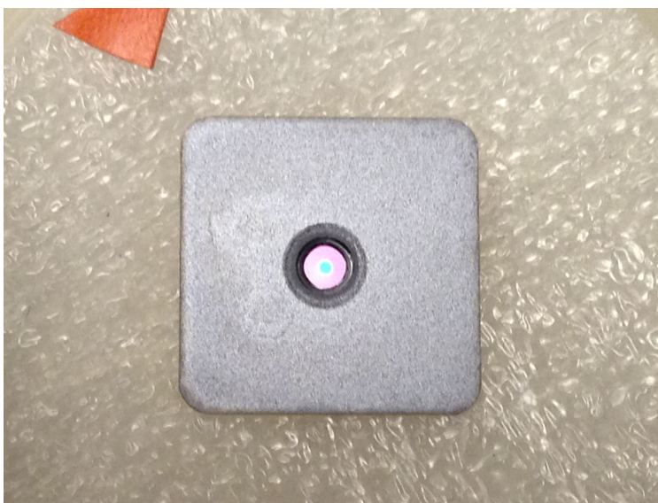
Figure 2.3: A photo of the diamond membrane on the silicon frame. The orange tape is for keeping track of the alignment corner
