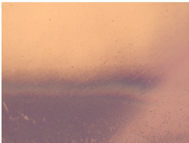
Figure 2.10: Microscope photograph of edge of diamond following deposition. Note the black burning and rainbow thin film interference bleeding into the deposited gold.
