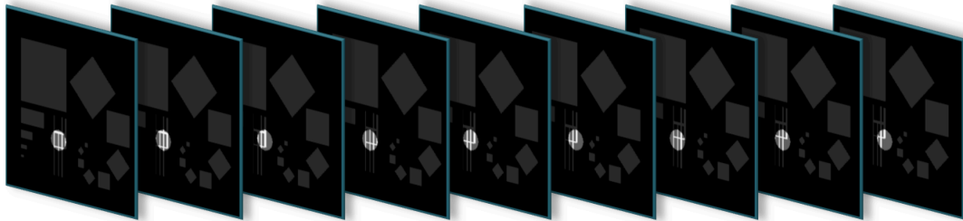
Figure 8: Cascading images of the exit wave amplitudes from a 3 \times 3 scan grid. These images show the exit waves from a ptychography simulation. The dark gray regions indicate the non-illuminated object, the light gray regions indicate the illuminated area where the object is opaque, and the white regions indicate the actual exit wave.
