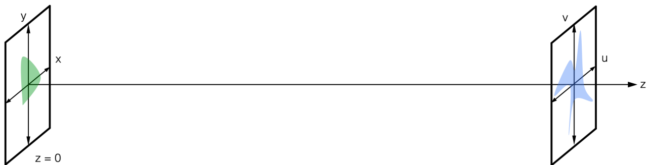
Figure 2: Visualization of the Fraunhofer diffraction equation. The plane with a green profile is the sample space where the probe illuminates the sample. The plane with a blue profile is the diffraction space which is necessarily far from the sample plane satisfying the far-field limit z \gg \frac{k}{2} (x^2 + y^2) .
