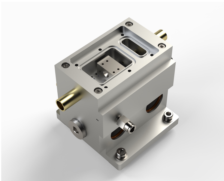
Figure 5.10: The full HHG source assembly on the pedestal, as it appears on the optical table. The large ports on the bottom of the pedestal connect to two roughing-level vacuum pumps. The lid is not pictured. Position registration of the chassis is ensured by a lip on the near side of the pedestal. In the configuration which generated harmonics, a window was epoxied to the brass laser entrance port insert; the backside insert is connected to the beamline with an ultraTorr fitting.
