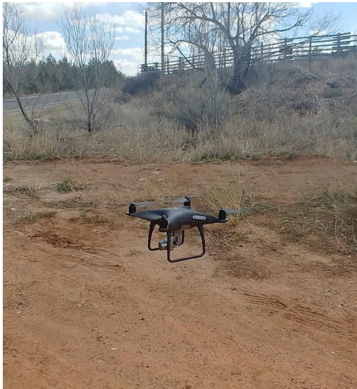
Figure 3: DJI Phantom 4 Drone used in imaging the April 1, 2019 flight of the Lyons study site.
