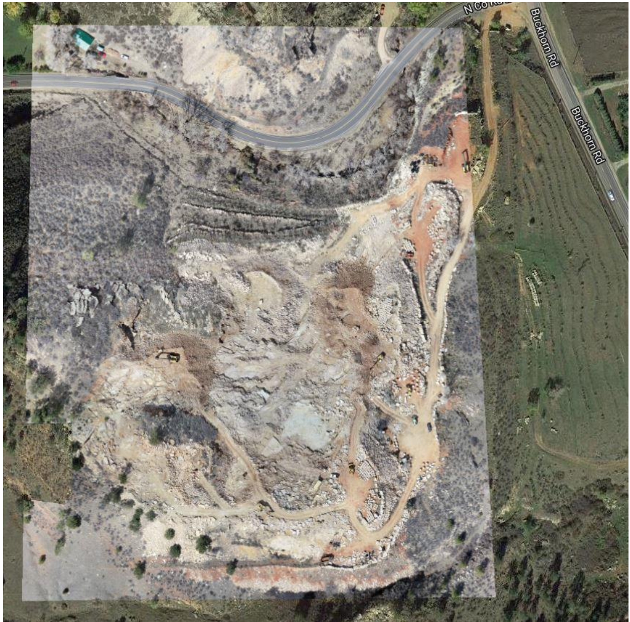
Figure 11: Orthomosaic of the drone imagery collected over the Lyons study site. This image was taken at an altitude of 400 ft above ground level (AGL) using a DJI Phantom 4 drone and 12 MP sensor. Imagery taken on April 1, 2019.
