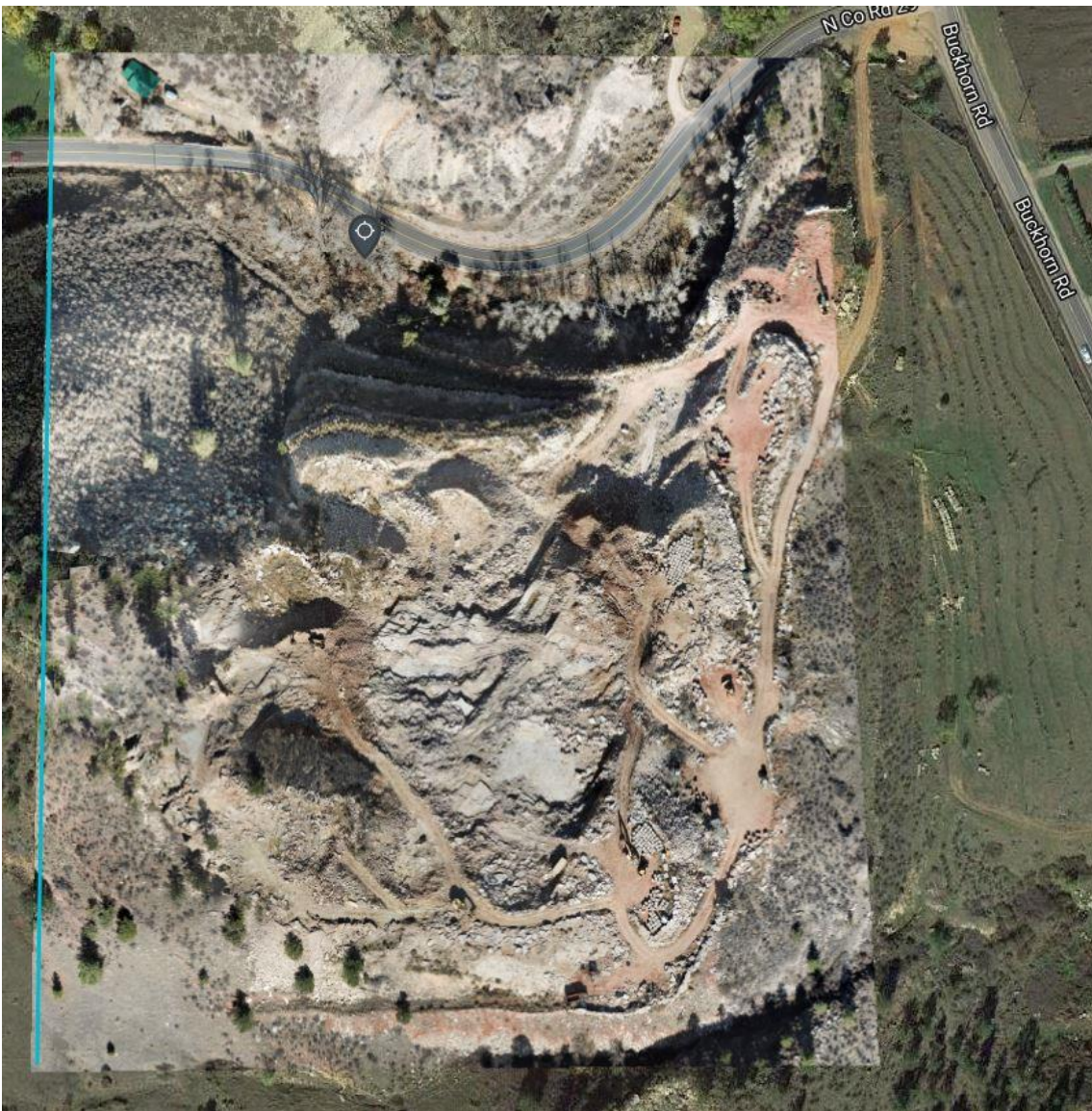
Figure 10: Orthomosaic of the drone imagery collected over the Lyons study site. This image was taken at an altitude of 400 ft above ground level (AGL) using a DJI Mavic Pro drone and 12 MP sensor. Imagery taken on November 10, 2018.
