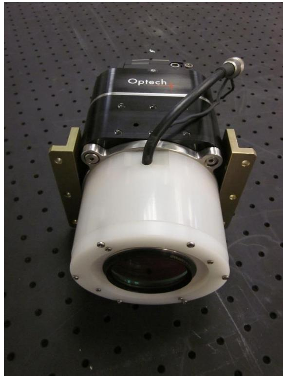
Figure 8: Optech DiMAC D8900 high spatial-resolution digital camera
