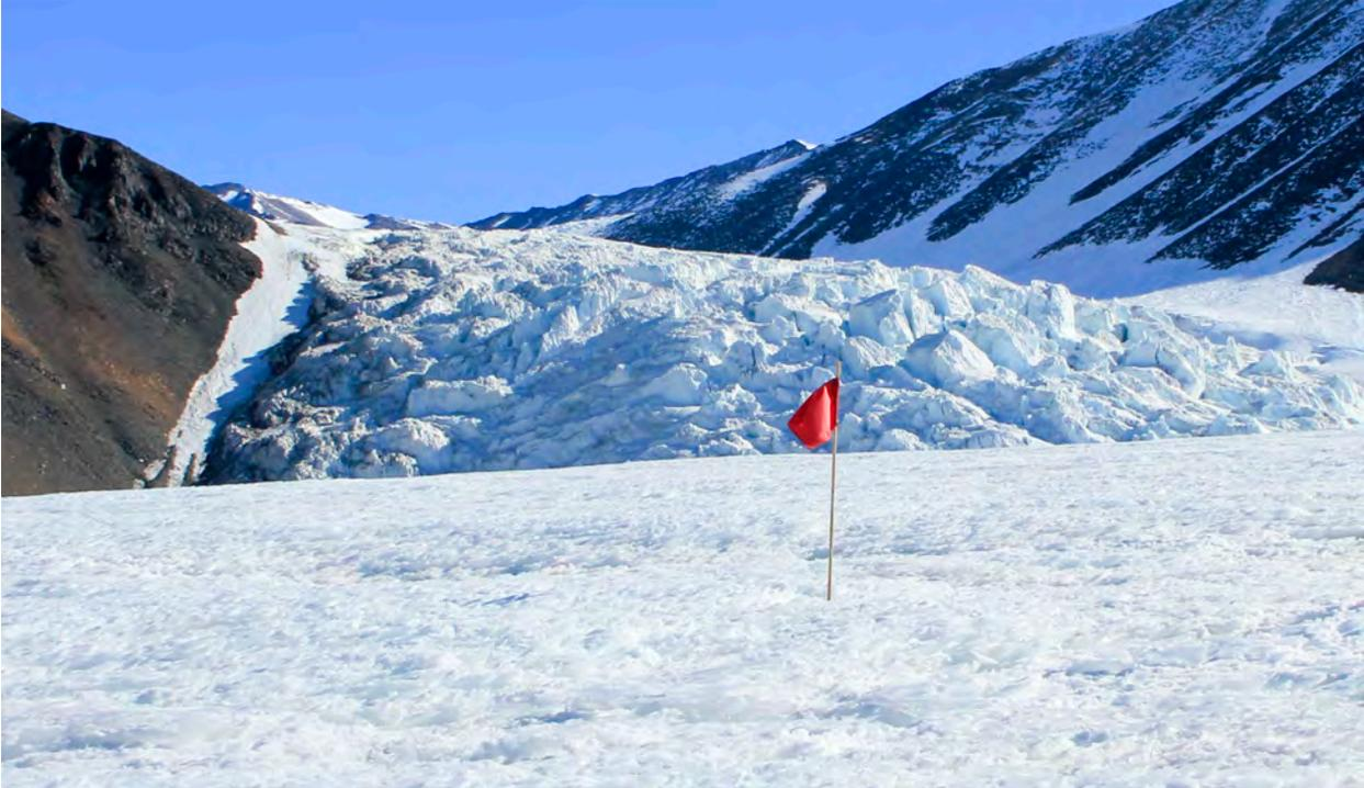
**Figure 3.2- Ablation stake on Canada Glacier.** *This bamboo post was drilled into the glacial surface and protrudes ~1m above the ice.*
