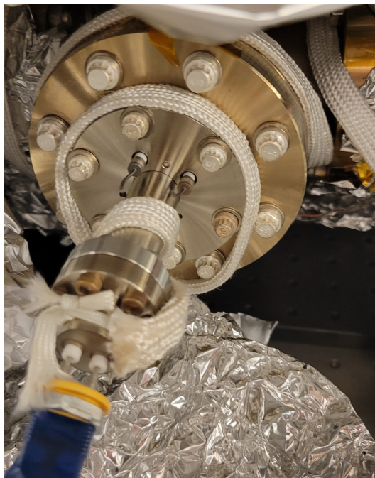
Figure 3.1: Sadly, the only picture I have depicting the heat wraps and foil, Specifically, the heat wraps are covering the end of the oven with the foil in the background covering the viewports.
