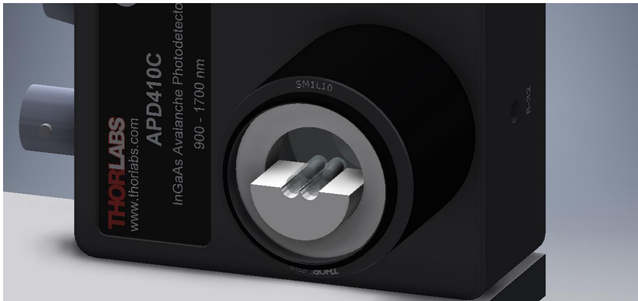
Figure 110: Light enters the detector from two GRIN/fiber assemblies. One path is the “online” wavelength, one is the “offline” wavelength. An aspheric lens focuses the light from both optics onto the detector. The GRIN/fiber assemblies are mounted on a 1” diameter part that threads into an optic tube mounted directly to the detector for maximum stiffness.
