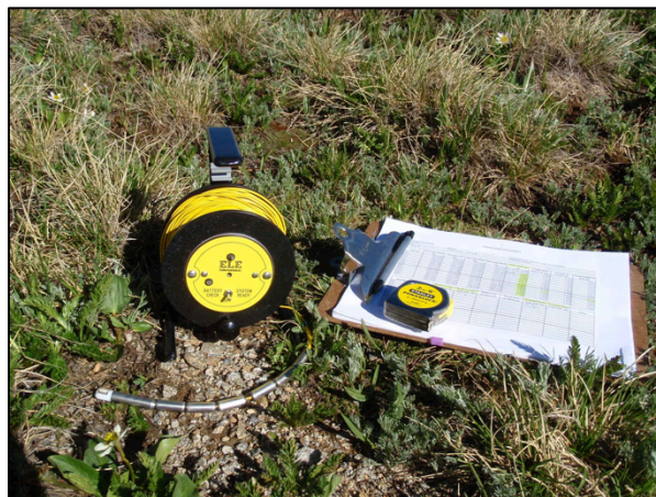
Figure 3.3. ELE International electrical water level indicator. Weekly to monthly water level measurements were made with either an electronic water level indicator or weighted tape.
