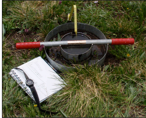
Figure 3.14. Double-ring infiltrometer used in this study. A tape measure affixed to the inside of the inner ring was used to measure the level of the ponded water. A stopwatch was used to measure the change in water level over time.
