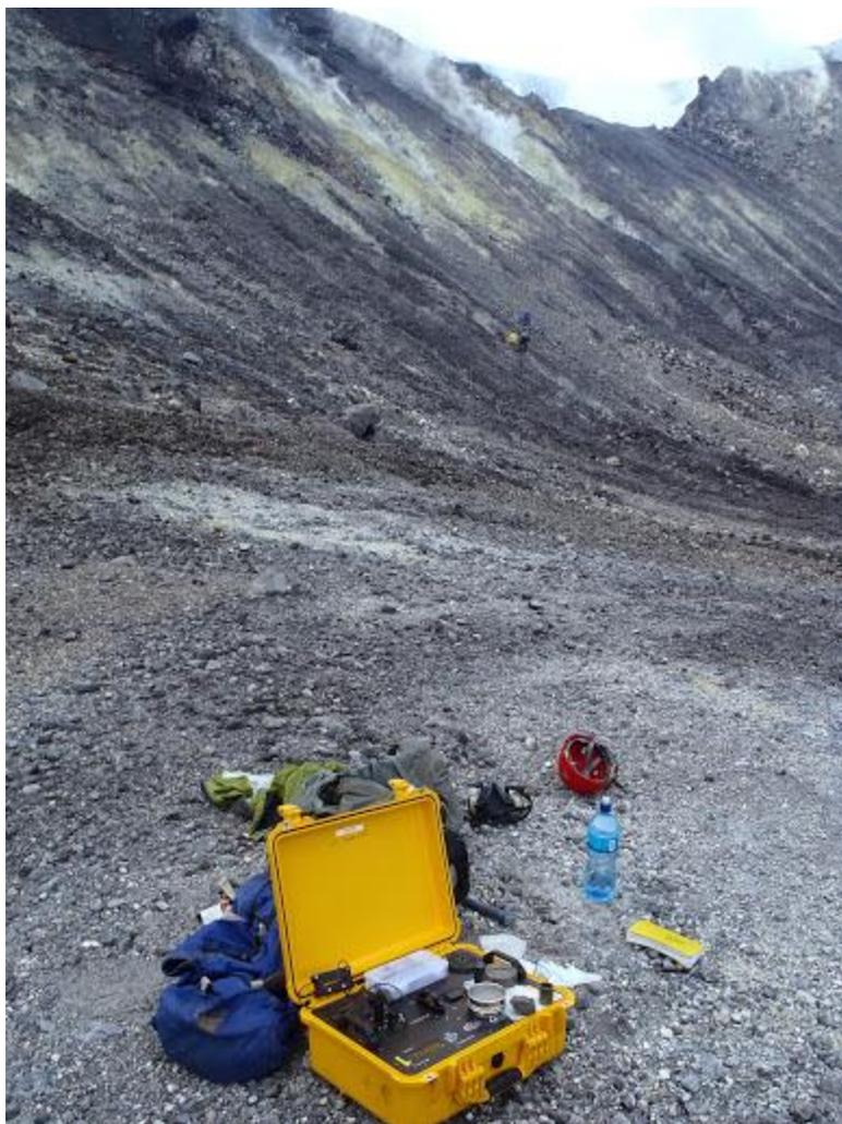
Figure 2.5: The Terra X-ray diffraction/X-ray fluorescence (XRD/ XRF) instrument in use near the Turritop site (near top of photo) and the center crater (out of frame to right).
