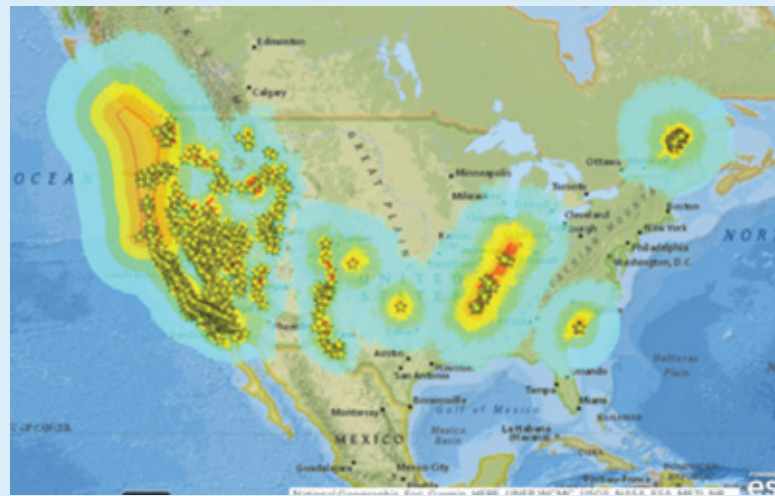
Figure 5. An authoritative map of ground shaking in realistic future earthquake scenarios. Each star indicates the epicenter of one such scenario. Warmer colors indicate stronger shaking in one of the maps. USGS, 2014 Building Seismic Safety Council (BSSC) Catalog , https://earthquake.usgs.gov/scenarios/catalog .
