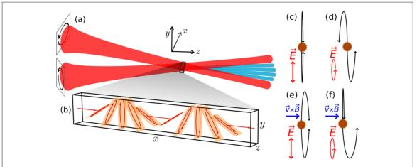
**Figure 1.** Two non-collinear circularly polarized beams (a) produce a polarization gradient across their focus in the transverse direction (b), including points with forwards ellipticity. This takes the usual linear trajectories (c) on a path to miss the ion (d), cancelling out the effect of the Lorentz force (e) to achieve one recollision per cycle (f), re-enabling the harmonic emission.
