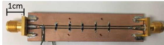
Figure A.2: 500 MHz to 1000 MHz input frequency NLTL fabricated with Skyworks SMV1247 diodes. The diode spacing is 7.7 mm, input power is 24 dBm, and reverse bias is 3.2 V.
