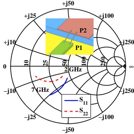
Figure 2.11: Simulated  $S_{11}$  and  $S_{22}$  versus frequency from 2 GHz to 7 GHz. The transformation from plane  $P_1$  to  $P_2$  depicted in Fig. 2.10 is significant and must be accounted for in order to present harmonic terminations at the virtual drain. Additionally, the impact of the transformation increases with frequency.
