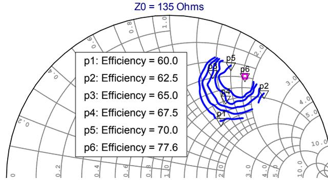
Figure 5.4: Source-pull contours at  $f_0$  with available input power to the diode set to 6 dBm. The  $2f_0$  and  $3f_0$  harmonics were terminated in short circuits. The impedance is referenced to the junction capacitance of the diode, therefore the lead inductance of the package has been compensated for. Setting  $R_{DC}$  to  $1080\ \Omega$  was found to result in the optimal efficiency for this input power.
