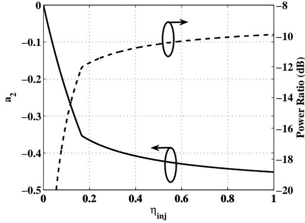
Figure 6.5: Optimal solution for Fourier coefficient  $a_2$  (solid line) and second harmonic delivered power relative to fundamental frequency output power (dashed line) versus second harmonic injection efficiency  $\eta_{inj}$ .
