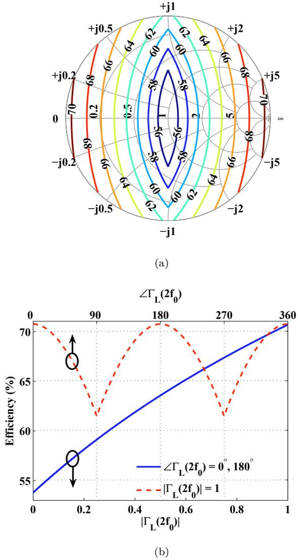
Figure 3.4: (a) Ideal second harmonic PA efficiency contours vs.  $z_L(2f_0)$ . The minimum efficiency of 53.76% occurs when  $z_L(2f_0) = 1$ . The maximum efficiency of 70.71% occurs when  $z_L(2f_0) = 0$  or  $z_L(2f_0) = \infty$ . (b) Ideal second harmonic PA efficiency for purely resistive and purely reactive  $z_L(2f_0)$ . The fundamental frequency impedance  $z_L(f_0)$  is purely real.
