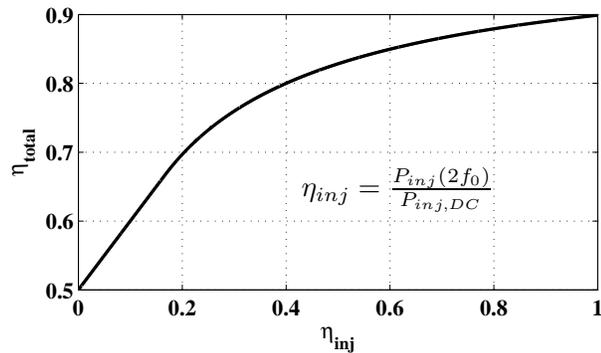
Figure 6.6: Total efficiency  $\eta_{total}$  versus injector efficiency  $\eta_{inj}$ .
