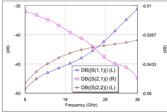
Figure 2.18: AXIEM<sup>®</sup> simulation of RF probe pad layout. Minimal parasitics are realized up to 36 GHz, which was chosen as the highest simulation frequency because it is the third harmonic of the highest X-band frequency (12 GHz).
