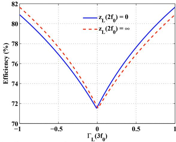
Figure 3.11: Ideal PA efficiency with fixed second harmonic versus  $\Gamma_L(3f_0)$  when  $\Gamma_L(3f_0)$  is purely real. Greater than 81% efficiency is achieved when  $\Gamma_L(3f_0) \geq +0.9$  for  $z_L(2f_0) = 0$  and  $\Gamma_L(3f_0) \leq -0.9$  for  $z_L(2f_0) = \infty$ . The minimum efficiency of 71.52% occurs when  $z_L(3f_0) \simeq z_L(f_0)$ . The fundamental frequency impedance  $z_L(f_0)$  is purely real.
