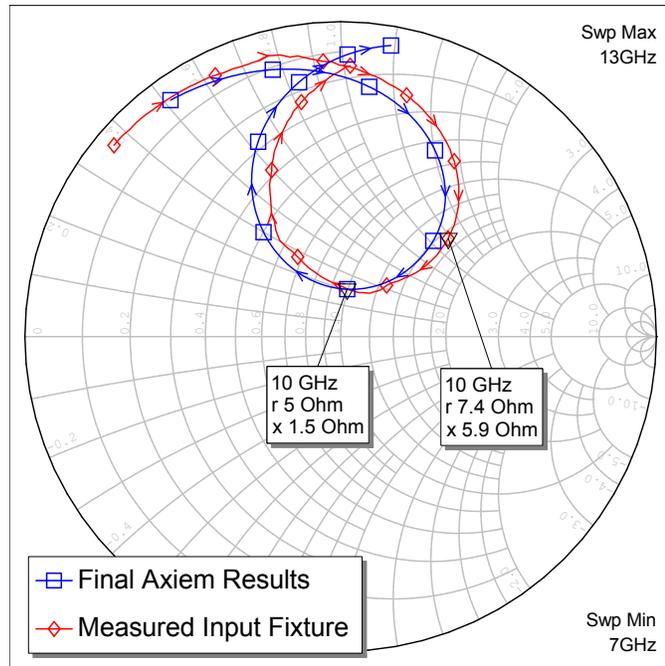
Figure 2.37: Simulated versus measured input pre-matching fixture impedance match. The measured results are slightly shifted in frequency relative to the simulation. The Smith Chart is normalized to  $5\ \Omega$ .
