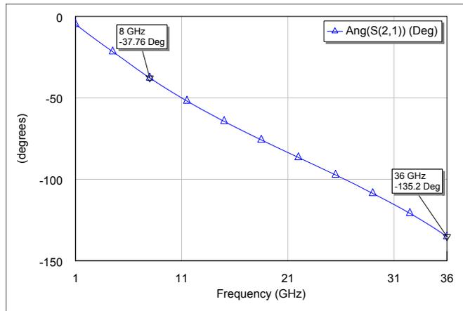
Figure 2.23: 300 μm line width TRL kit line phase simulated with AXIEM<sup>®</sup>. The phase is well within the recommended range of 30° - 150° over the frequency range 8 GHz - 36 GHz.
