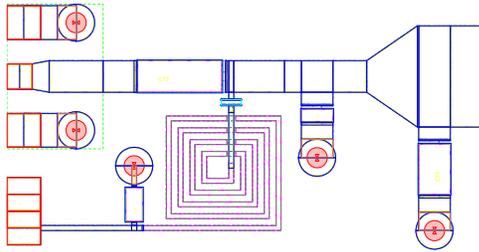
Figure 2.27: Input matching circuit with bias tee layout.
