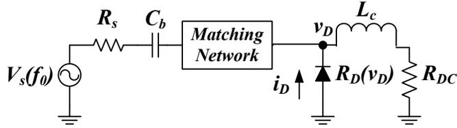
Figure 5.1: Microwave rectifier circuit diagram. An ideal blocking capacitor  $C_b$  provides dc isolation between the microwave source and rectifying element. An ideal choke inductor  $L_c$  isolates the dc load  $R_{DC}$  from RF power.
