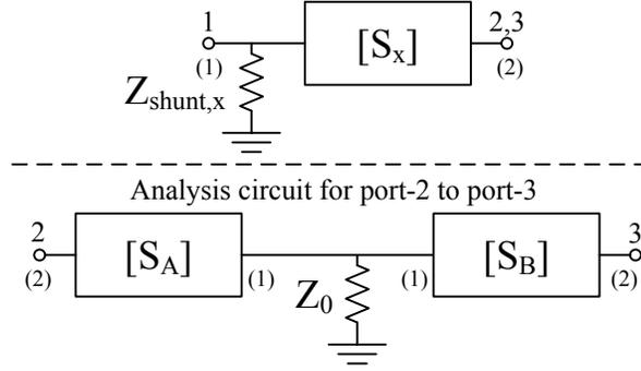
Figure 6.13: Diagram showing the circuits used to determine the three-port scattering parameters.  $Z_{shunt,x}$  and  $[S_x]$  denote a shunt impedance and scattering parameter block, respectively. Note that in general  $Z_{shunt,x}$  and  $[S_x]$  will differ for each analysis circuit. For example,  $Z_{shunt,x}$  and  $[S_x]$  will differ for the analysis of port-1 to port-2 and port-1 to port-3, although they are represented by the same basic circuit in the figure.
