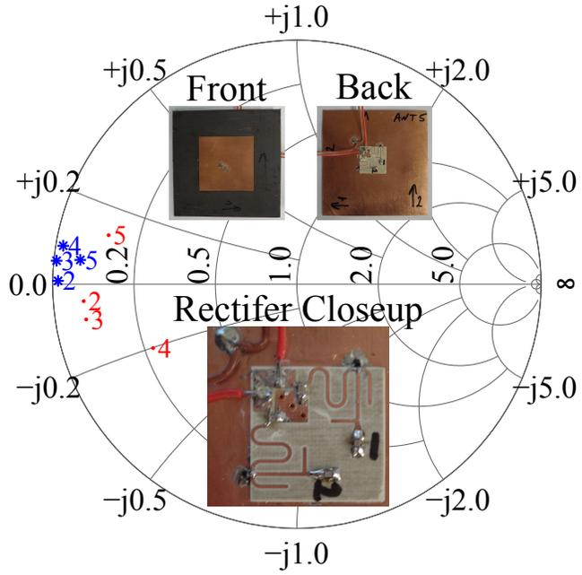
Figure 5.6: Dual-linearly polarized patch rectenna and associated  $2f_0$ - $5f_0$  terminations ( $50\ \Omega$  Smith Chart) [2]. Blue and red indicate the simulated and measured harmonic terminations, respectively. The rectifiers are dc isolated.
