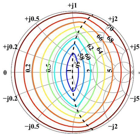
Figure 3.12: Ideal PA efficiency contours vs.  $z_L(2f_0)$  when the normalized load reactance  $x_L(f_0)$  is optimized in addition to the harmonic Fourier coefficients. The minimum efficiency and maximum efficiency are equivalent to those calculated without optimizing  $x_L(f_0)$ . However, the regions for which a given high efficiency is obtained are significantly expanded.
