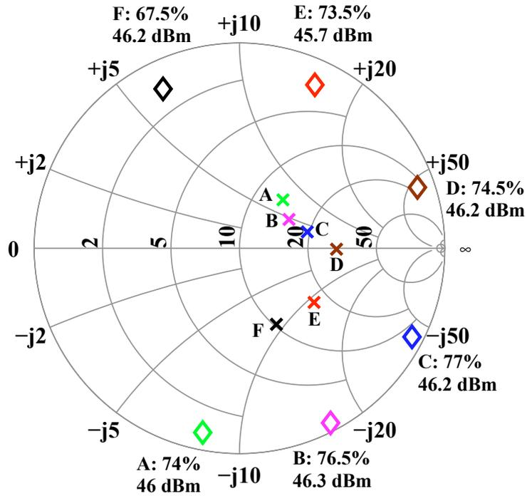
Figure 3.21: Results from harmonic load pull of Triquint 50 W device on a 10  $\Omega$  Smith Chart. The points denoted by diamonds mark the second harmonic termination at the virtual drain along with resultant peak drain efficiency and associated fundamental output power. The points denoted by an x mark the fundamental load impedance resulting in peak drain efficiency for each respective second harmonic termination.
