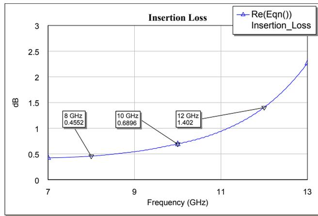
Figure 2.34: Insertion loss of the output matching circuit.
