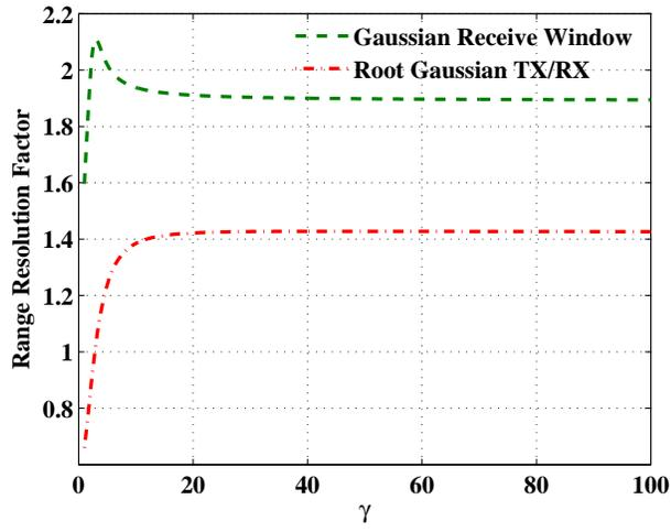
Figure 4.5: Range resolution factor versus time-bandwidth product  $\gamma$  for 4 dB PAR Gaussian window either full applied on receive or split on transmit and receive. The results are normalized to the range resolution achieved when a un-weighted LFM pulse is processed with its matched filter.
