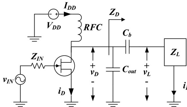
Figure 3.17: Circuit diagram of ideal common source FET-based PA with incorporation of a constant output capacitance  $C_{out}$ . The S-parameters of  $C_{out}$  represent a transformation between the virtual drain and the measurable plane corresponding to the loading network  $Z_L$ .
