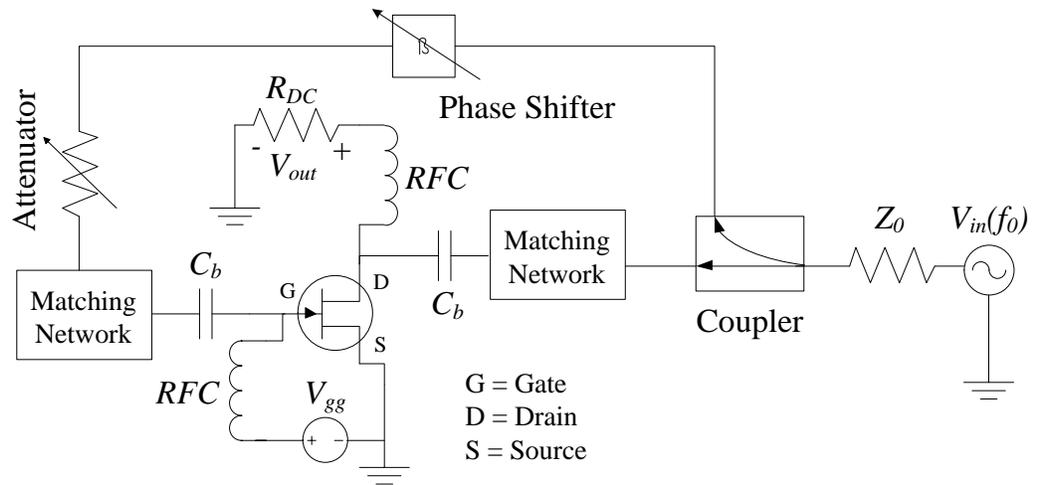
Figure 7.1: Transistor rectifier block diagram. The fundamental frequency RF source shown as  $V_{in}(f_0)$  and  $Z_0$  is used to drive both the drain and the gate of the field effect transistor in a common source configuration.
