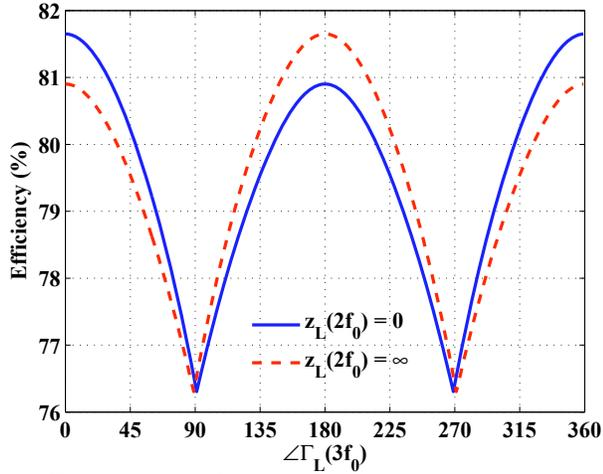
Figure 3.10: Ideal PA efficiency with fixed second harmonic versus  $\angle\Gamma_L(3f_0)$ ,  $|\Gamma_L(3f_0)| = 1$ . Greater than 81% efficiency is achieved within  $\pm 30.0^\circ$  of the ideal termination. The fundamental frequency impedance  $z_L(f_0)$  is purely real.
