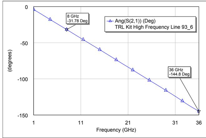
Figure 2.21: 50 Ω TRL kit line phase simulated with AXIEM<sup>®</sup>. The phase is well within the recommended range of 20° - 160° over the frequency range 8 GHz - 36 GHz [1].
