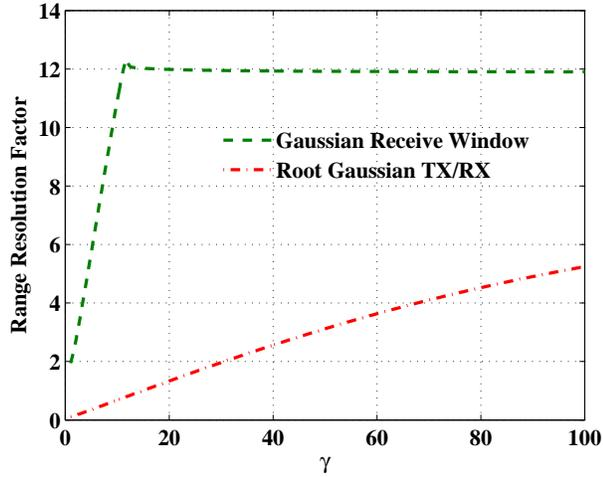
Figure 4.7: Range resolution factor versus time-bandwidth product  $\gamma$  for 12 dB PAR Gaussian window either full applied on receive or split on transmit and receive. The results are normalized to the range resolution achieved when a un-weighted LFM pulse is processed with its matched filter.
