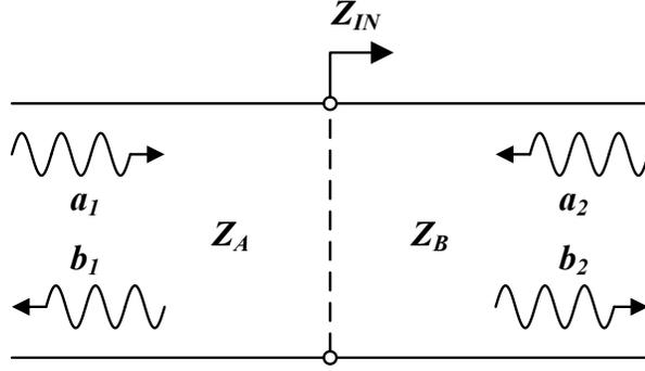
Figure 6.1: Basic impedance synthesis circuit depicting two simultaneous excitations.
