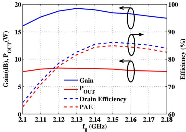
Figure 2.15: Measurements of transducer gain, delivered output power, drain efficiency and PAE versus frequency at  $V_{DD} = 34$  V. Peak PAE of 84.9% occurs at 2.15 GHz. The amplifier exhibits over 70% peak PAE, 7.8 W output power, and 17.7 dB gain over the entire 2.11 - 2.17 GHz W-CDMA bandwidth. For most of the W-CDMA bandwidth, the peak PAE exceeds 80%.
