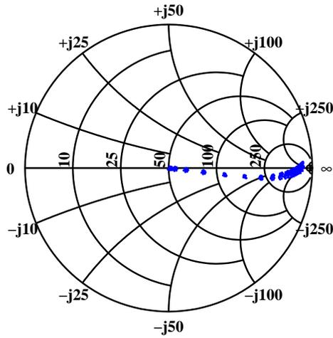
Figure 2.5: Initial measured points following phase normalization.
