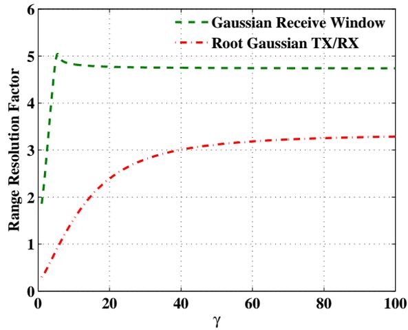
Figure 4.6: Range resolution factor versus time-bandwidth product  $\gamma$  for 8 dB PAR Gaussian window either full applied on receive or split on transmit and receive. The results are normalized to the range resolution achieved when a un-weighted LFM pulse is processed with its matched filter.
