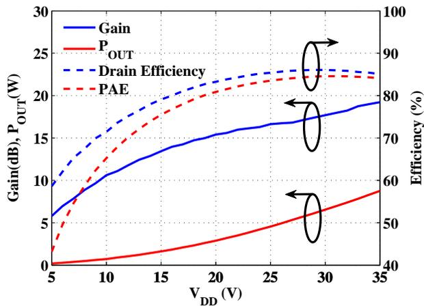
Figure 2.14: Measurements of transducer gain, delivered output power, drain efficiency and PAE at 2.14 GHz. Peak 2.14 GHz PAE of 84.6% occurs at  $V_{DD} = 31$  V, having 7 W output power, 18 dB Gain, and 86% drain efficiency.
