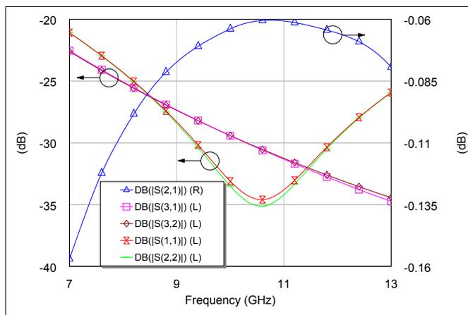
Figure 2.25: Gate bias tee relevant scattering parameters.
