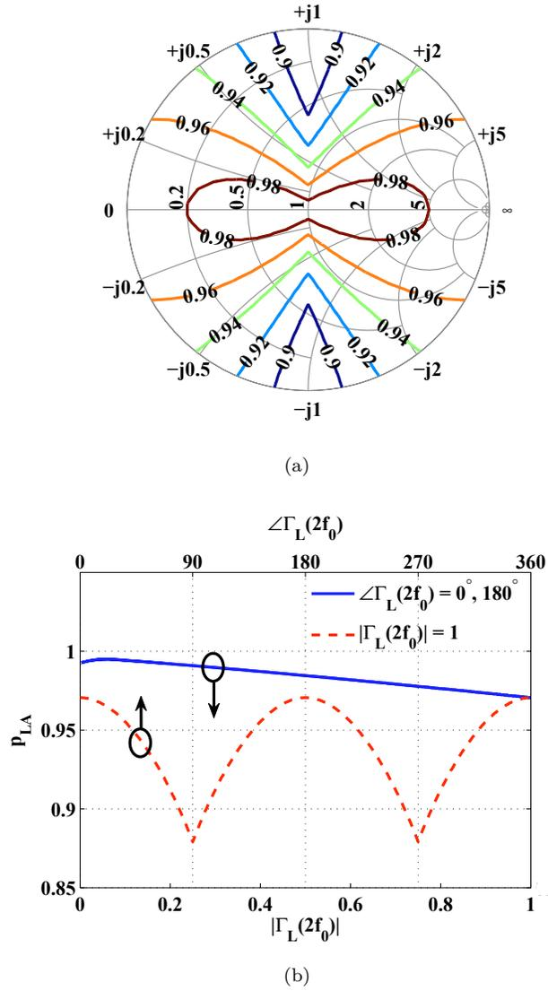
Figure 3.5: (a) Ideal second harmonic PA normalized power  $p_{LA}(f_0)$  contours vs.  $z_L(2f_0)$ . (b) Ideal second harmonic PA  $p_{LA}(f_0)$  for purely resistive and purely reactive  $z_L(2f_0)$ . The fundamental frequency impedance  $z_L(f_0)$  is purely real.
