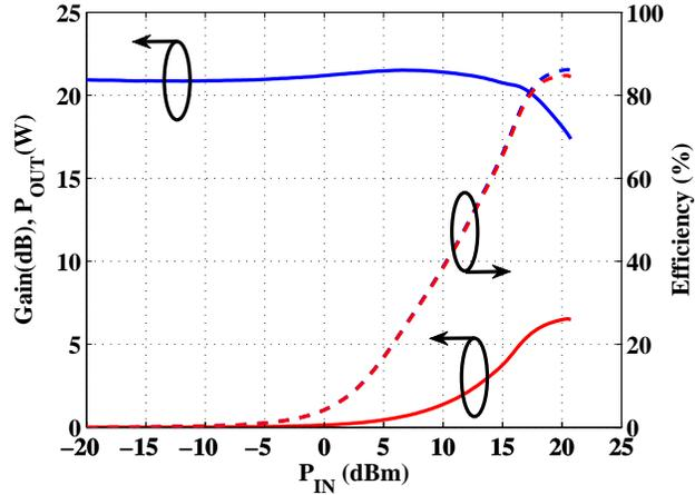
Figure 2.13: Measured PA performance at design point of 2.14 GHz versus input power,  $V_{DD} = 30$  V. The gain undergoes a slight expansion from 21.0 dB to 21.5 dB prior to entering compression. A peak PAE of over 84% is realized at the 3.6 dB gain compression point, corresponding to 20.2 dBm input power and 6.5 W output power at the design point.
