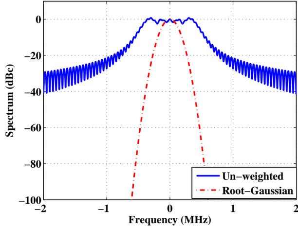
Figure 4.1: Example of un-weighted transmit spectrum versus root Gaussian Weighted transmit spectrum resulting in 8 dB PAR. The time-bandwidth product  $\gamma$  was set to 20, with the swept bandwidth  $B$  set to 1 MHz.
