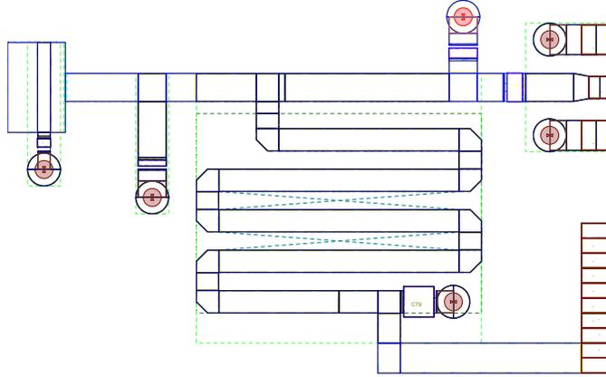
Figure 2.33: Layout of output matching circuit. The far left connects to the transistor drain.
