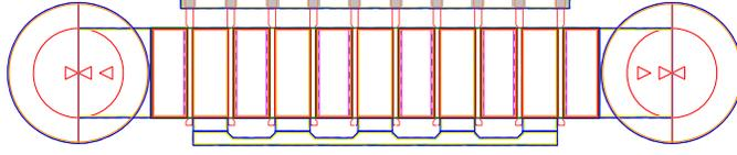
Figure 2.19: Active device selected for load pull measurement. The gate is the top side, with the drain being the bottom side. The circular structures are substrate vias. The device has a  $70 \mu\text{m}$  gate width with 10 gate fingers, corresponding to  $700 \mu\text{m}$  of gate periphery.
