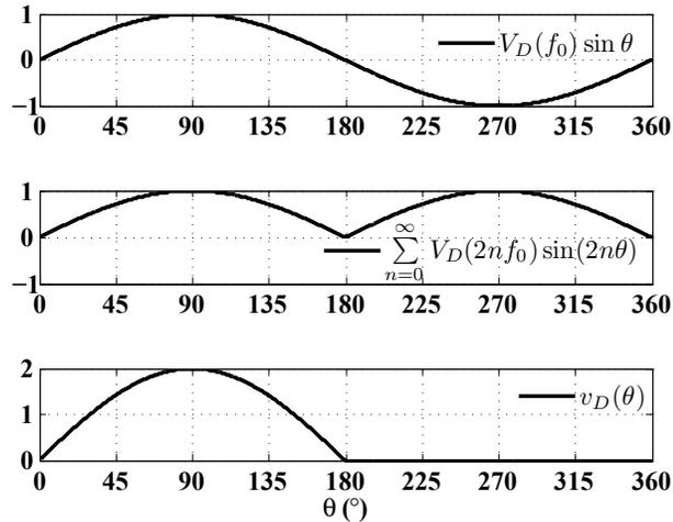
Figure 5.11: Class-F<sup>-1</sup> half-wave rectifier voltage waveform construction. The voltage is normalized to  $v_D(f_0)$ .
