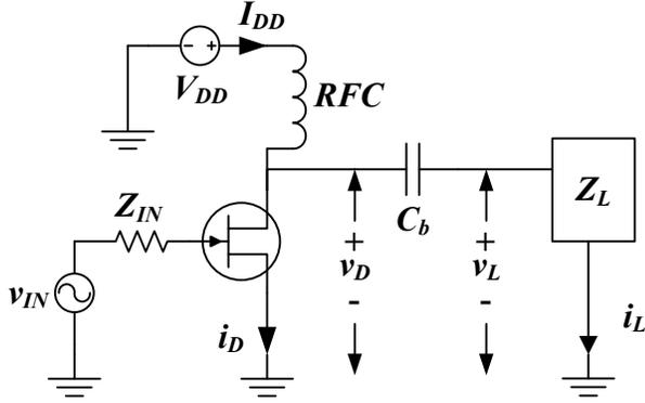
Figure 3.1: Circuit diagram of ideal common source FET-based PA. The DC Block ( $C_b$ ) and RF Choke (RFC) are assumed to be ideal, therefore  $Z_L$  is equivalent to the impedance  $Z_D$  presented to the virtual drain at the fundamental and harmonic frequencies.
