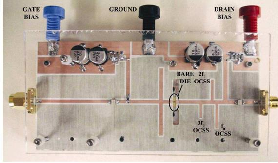
Figure 2.12: Photo of prototype amplifier. Note that no tuning of the amplifier was required to achieve the presented performance. Bias lines are implemented with  $\lambda/4$  transmission lines shorted to ground with resonant capacitors at 2.14 GHz. Several decades of capacitors (100 pF - 10  $\mu$ F) are implemented in the design to suppress low frequency oscillations. A 10  $\Omega$  series resistor on the gate bias line is used to improve stability.
