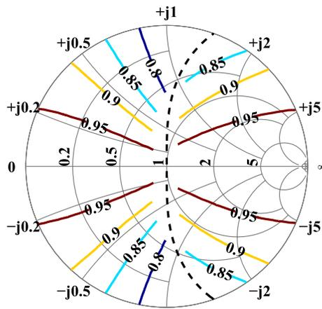
Figure 3.13: Ideal PA  $p_{LA}(f_0)$  contours vs.  $z_L(2f_0)$  when  $x_L(f_0)$  is optimized in addition to the harmonic Fourier coefficients. Power is reduced in order to improve efficiency for much of the Smith Chart. In the worst case, power is reduced by 1.63 dB relative to class-A output power.
