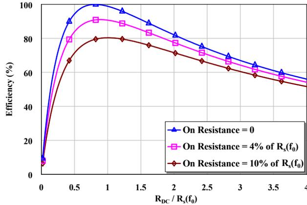
Figure 5.13: Simulated efficiency of class-F<sup>-1</sup> rectifier versus  $R_{DC}/R_s(f_0)$  for varying rectifier on-resistance.
