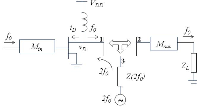
Figure 6.4: Block diagram of a linear PA with second harmonic injection at the virtual drain. The three-port network is an ideal passive injection circuit element described in Section 6.5 and further analyzed in Section 6.6. The injector voltage and impedance  $Z(2f_0)$  determine the dissipation in the transistor. The matching networks at input and output are designed for a linear PA.
