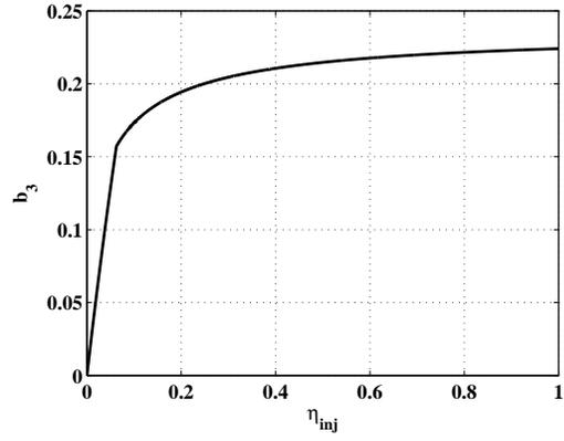
Figure 6.9: Solution for  $b_3$  versus injector efficiency.
