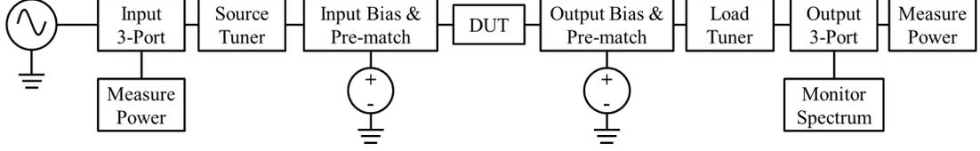
Figure 2.1: Basic fundamental frequency load pull block diagram.
