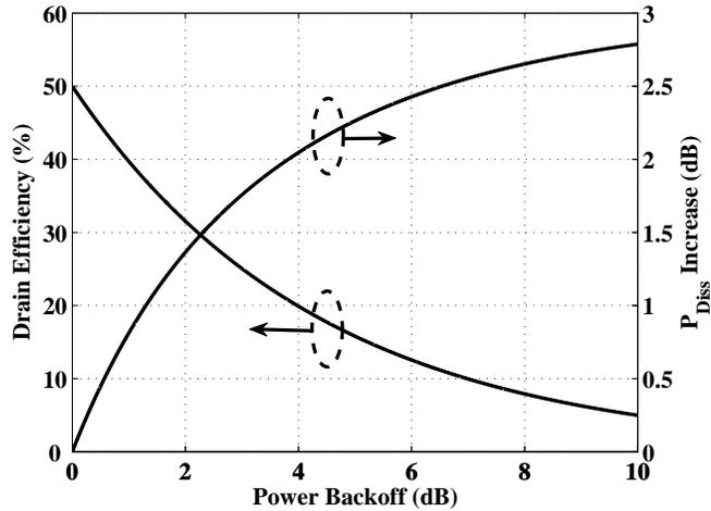
Figure 1.3: Class-A amplifier performance versus input power back-off.
