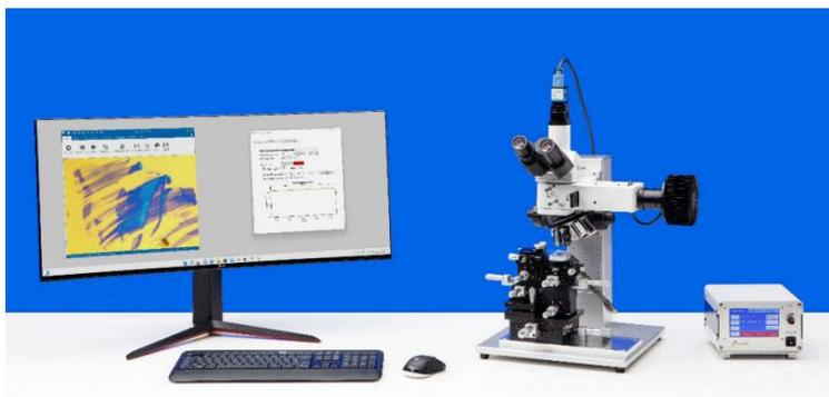
Figure 1.3: Photograph of a standard 2D materials transfer system setup. Image link: <https://www.hq2d.com/>
