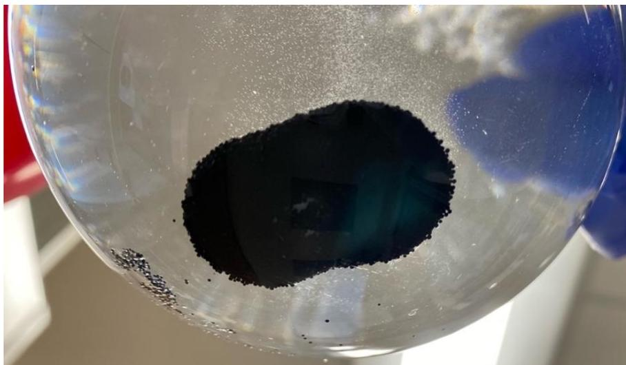
**Figure 36.** NZVI-A600E attracted to a metal stir bar in a round bottom flask.
