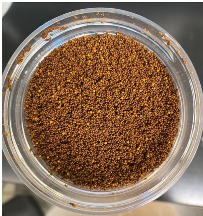
**Figure 18.** Purolite ArsenX<sup>np</sup> HIX resin.
