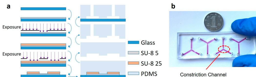
**Figure 2.** Fabrication process (a) and a prototype device (b) of the microfluidic module. In the microfluidic module, a micro device with a constriction channel was fabricated using conventional soft lithography including key steps of SU-8 exposure, PDMS molding and bonding between patterned PDMS with a glass slide.
