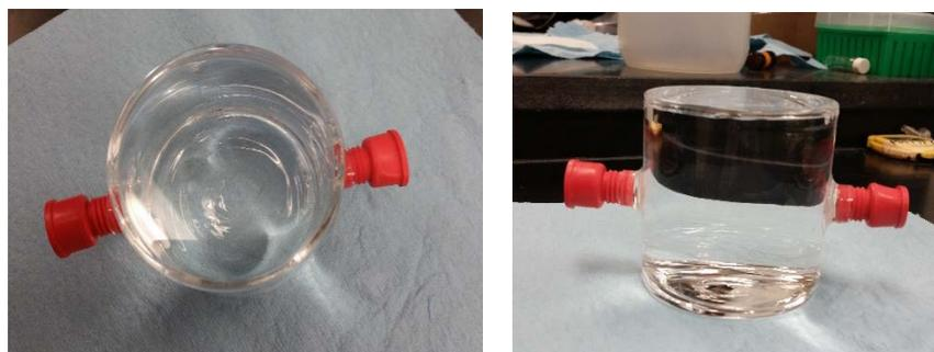
Figure 3: Quartz vessel customized for VOC samples
