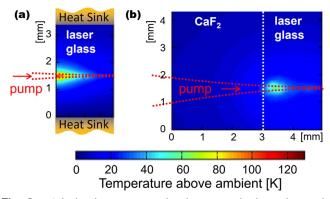
**Fig. 2.** Calculated temperature distribution in the laser glass under 500 mW pumping at 977 nm. (a) Traditional method: side-cooled laser glass. (b) Laser glass heat-sunk through the  $CaF_2$  cavity spacer. The  $CaF_2$  heat sink dramatically lowers the laser glass surface temperature from 117 K above ambient for side-cooled glass to only 32 K above ambient when cooled through the  $CaF_2$  spacer.
