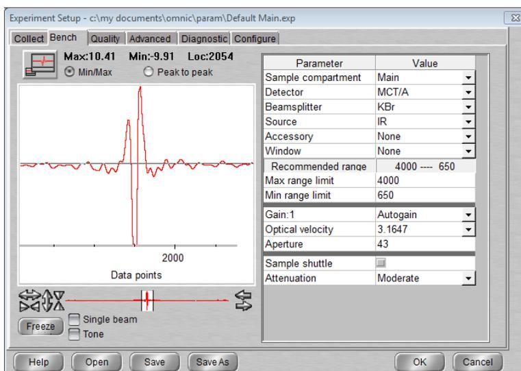
Figure 18: OMNIC experimental setup, bench page given with default parameters for experiment and proper interferogram depiction.
