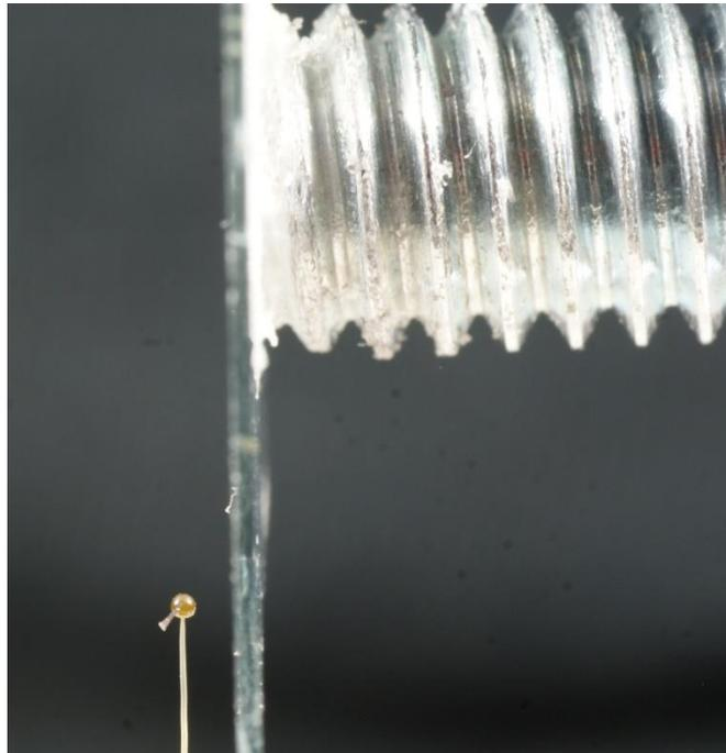
Figure 13: The above image depicts the setup used for the avoidance response. A microscopic slide attached to a threaded bolt is used as a barrier.
