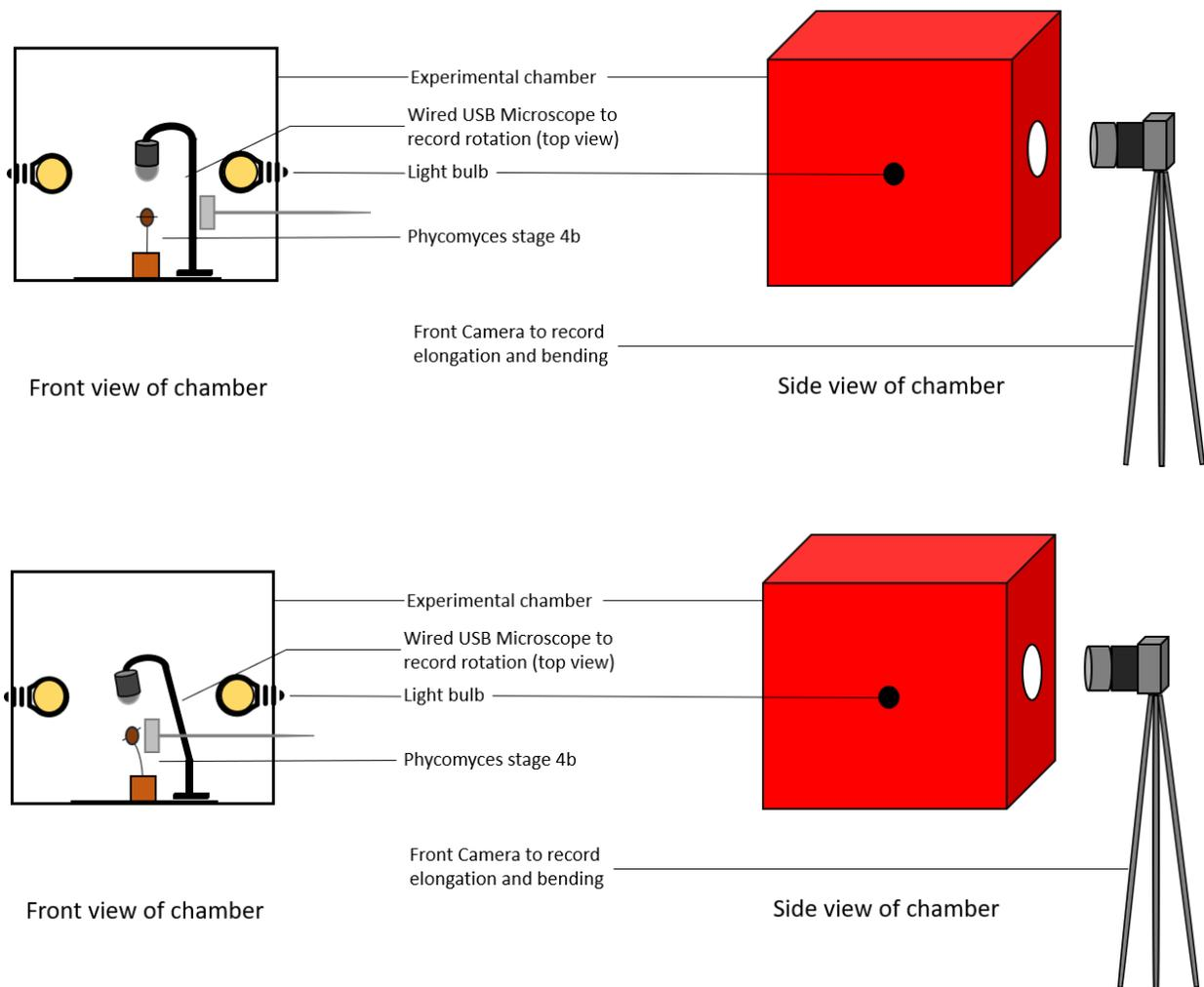
Figure 15: The diagram above depicts the experimental setup for conducting avoidance response experiments.
