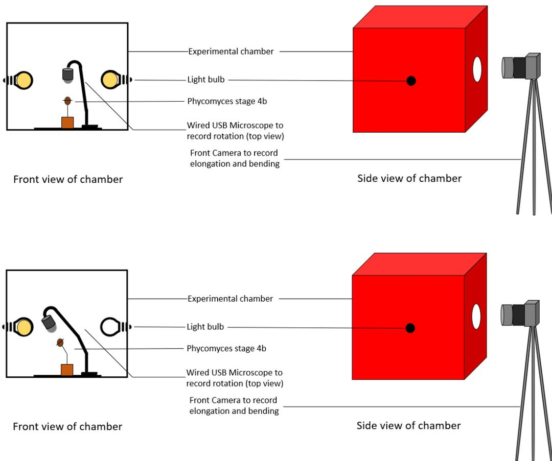
Figure 14: The diagram above depicts the experimental setup for conducting phototropic response experiments.
