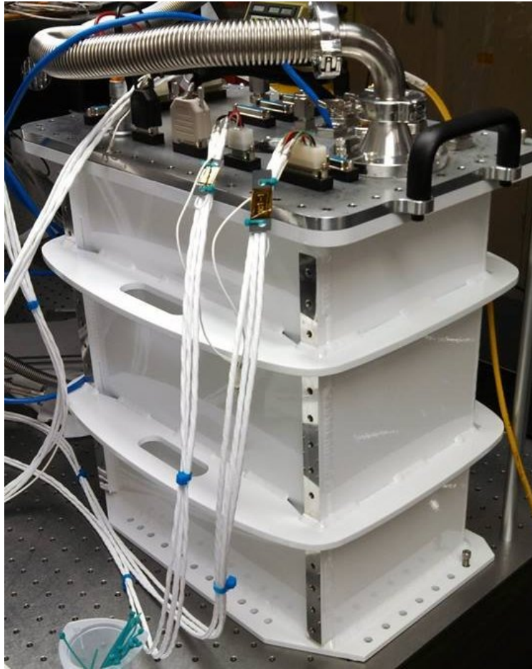
Figure 2.19: The ECS resides in a pressure vessel separate from the optics bench. This box has passthroughs that connect to the cameras, mechanisms and heaters. It also has ethernet and USB ports for programming and ground support communication.
