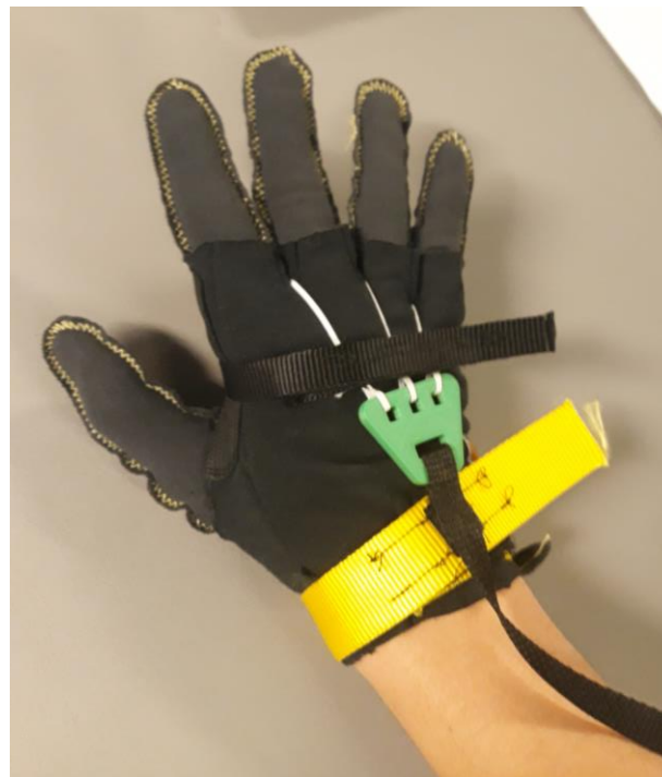
Figure 4.35. Anchoring Gauntlet v3. All elements have been integrated, including the 3D printed element.
