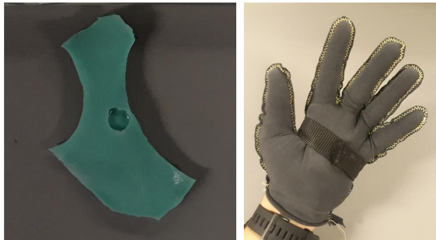
Figure 4.24. Palmar Pressure Distributor v1. The silicone hand mold is cut (left) and placed under the ERL, along a belt to help fix it on the palm.
