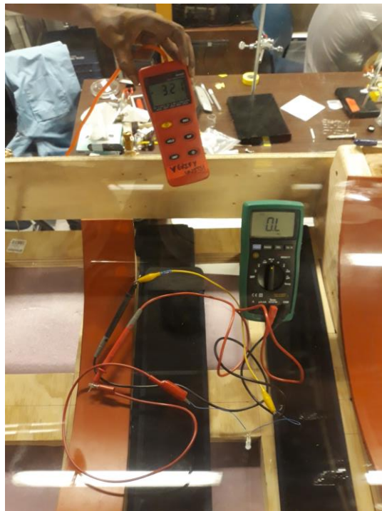
Figure A3.9. FSR Test Inside the Glovebox. The multimeter (green, front) connected to the FSR sensor (blue wires, front) displays a 0 value inside the glovebox, while the pressure reader (orange, back) shows that the glovebox has a 3.2psi environmental pressure
