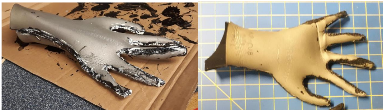
Figure 4.17. Elastic Restrain Layer v2. The left image it can be seen how the silicone-based layer (in white) is drying. The right image the final result can be seen.
