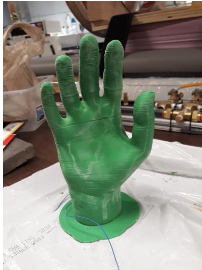
Figure A3.4. 3D Printed Hand Support. Finished 3D printed Hand support which, although being sanded, still shows some discontinuities over its surface due to the 3D printing technique used. However, the surface is smooth enough so that these discontinuities won't have any effect on the donning/doffing of the glove nor on the applied pressure sensing.
