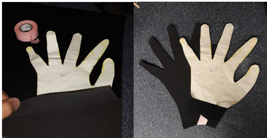
Figure 4.19. Definitive Neoprene Wetsudiving Pattern cut. The darkest side corresponds to the inner side of the MCP glove, as it is covered by spandex, which facilitates donning and doffing.
