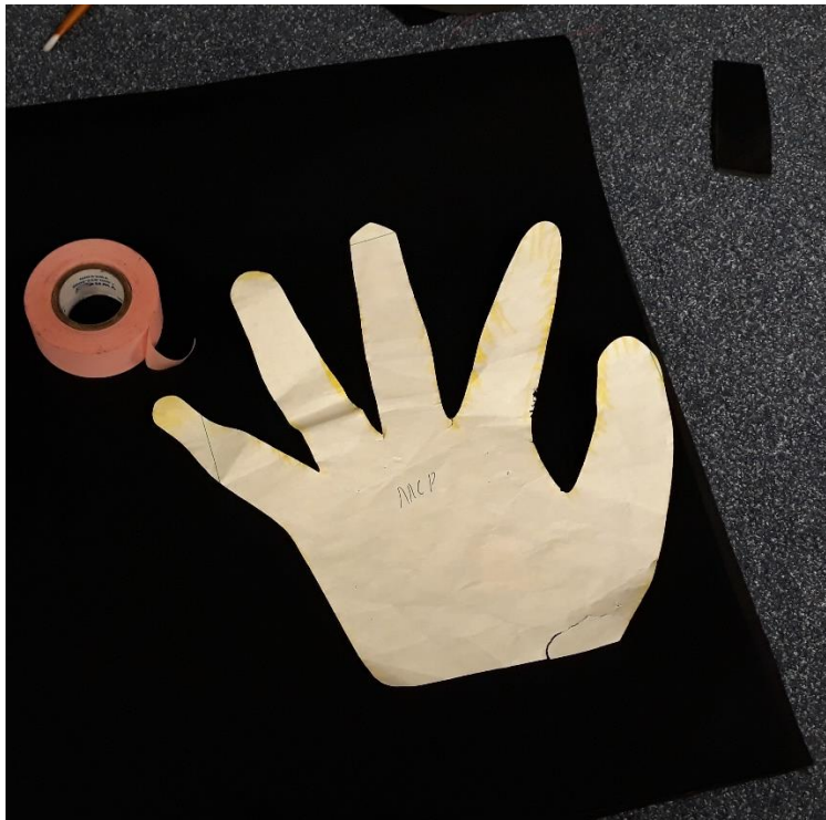
Figure 4.11. Laser cut paper with the MCP pattern. The fabric behind it is the Wetsuit Neoprene that is intended to be used for the MCP glove restrain layer.
