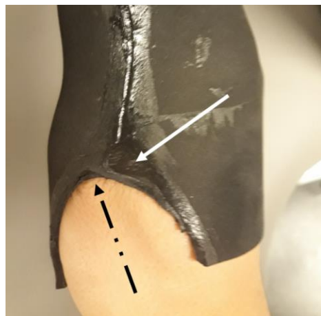
Figure 4.18. Neoprene Cement Break-Stress test. As it can be seen, the fabric breaks along the bond, but not through it (black arrow). Also, the elasticity of the neoprene cement that was used is marked by the white arrow.
