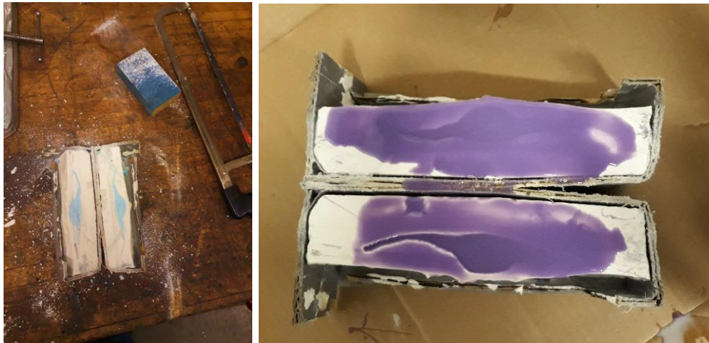
Figure 4.26. PPD Plaster Molt. On the left, the plaster model can be seen how has been cut in half with still the putty dough model still in it. On the right, the plaster mold has been emptied and filled with silicone.
