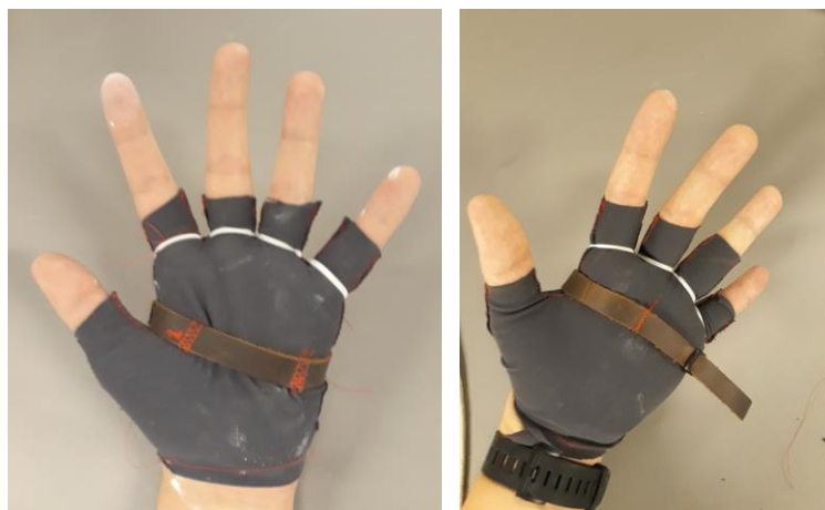
Figure 4.30. Study on the Palmar Central Restrain Anchoring. Two point seam in the left image. Single point anchoring seam in the right image.
