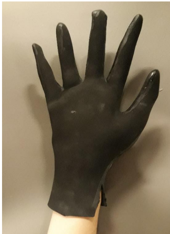
Figure 4.22. Elastic Restrain Layer v3. Without any thread used, the ERLv3 achieves the desired design characteristics, as it is completely flat in its inner side, has the exact coded pattern shape and applies a strong pressure on the fingers and most parts of the hand of its user.
