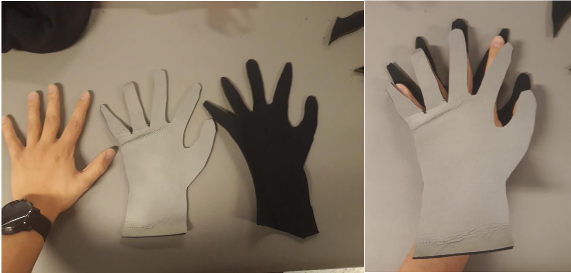
Figure 4.14. Thicker Wetsuit Neoprene. The two specular sides of the glove are depicted, showing that in for this material the neoprene side covered by spandex (in black) faces the inner part of the glove while the neoprene side covered with impermeable paint (in light grey) faces the exterior.
