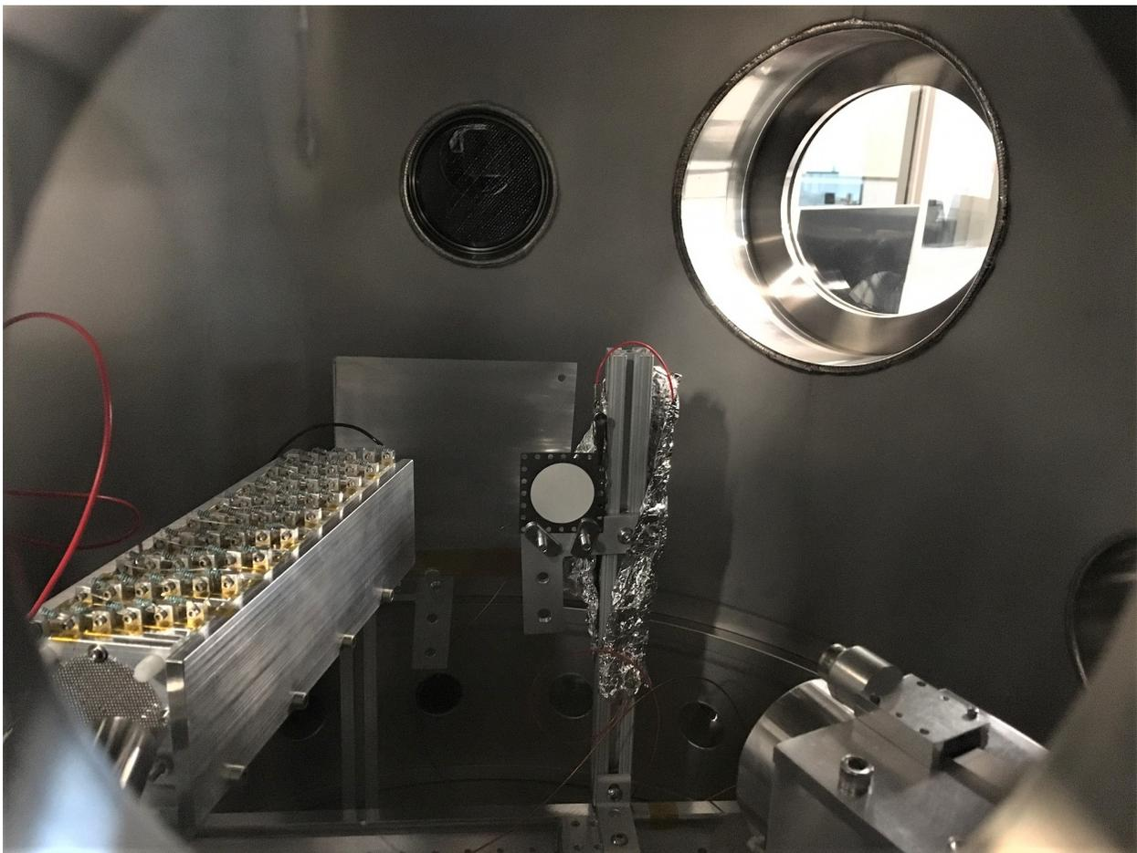
Figure 5.14: Setup for passive sensing experiment with the broad-spectrum electron gun. The broad-spectrum source is on the left, the target plate is at center, and the RPA is visible in the lower right.
