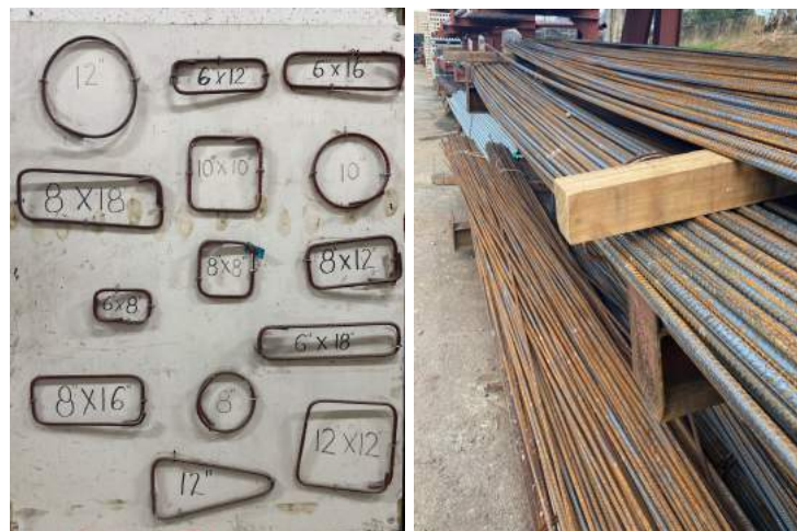
Figure 3.11: Steel reinforcing bars used in home construction. Transverse ties are sold in pre-defined bent shapes; the 6 x 12 in bars are most common. The most common longitudinal bars are no. 4 and no. 5, and are often stored outside (Humacao, Puerto Rico). [Photos: Polly B. Murray]
