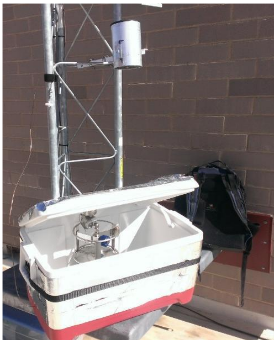
Figure S2. Typical field sampling set up. The adsorbent cartridge is in the inverted coffee can. The canister is in a cooler box.
