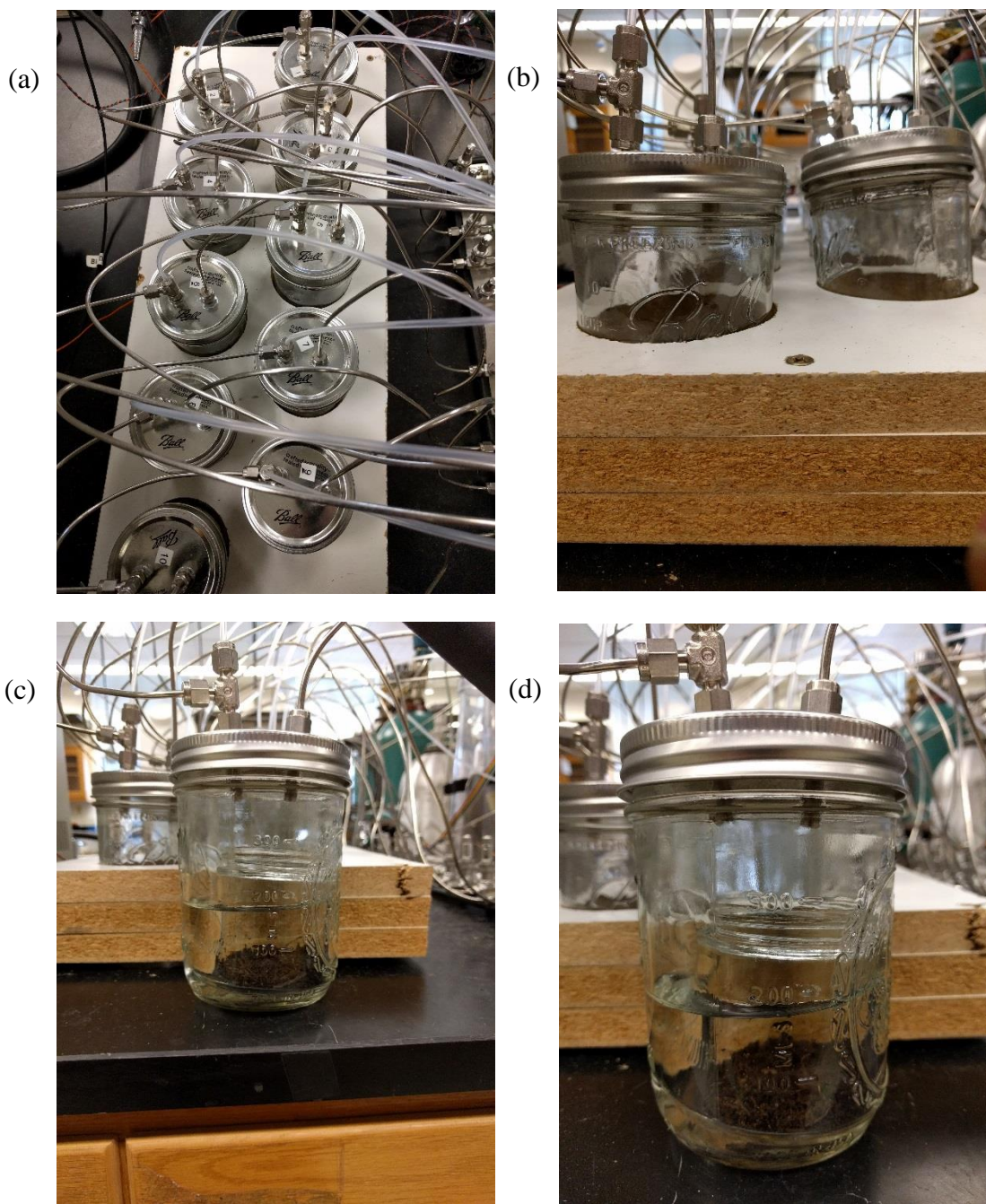
Figure S1. Photos of the dynamic flux chamber system. (a) Flux chambers from above. (b) The system from the side and shows the chambers in the manifold. (c) and (d) A chamber with a jar for soil and 50 mL of standing water to keep the humidity higher. Note that the soil in the photo was not used in this experiment, has not been homogenized or sieved, and only used to demonstrate the soil sampling set up.
