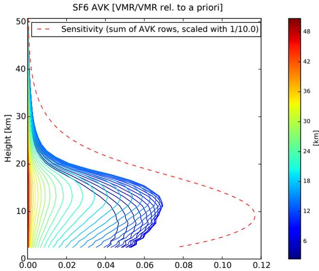
**Figure 3.** The typical averaging kernel of SF<sub>6</sub> retrieval at Maïdo. The solid lines represent the sensitivities at specific altitudes. The red dashed line is the sum of the rows of averaging kernels scaled by 0.1, indicating the vertical sensitivity.
