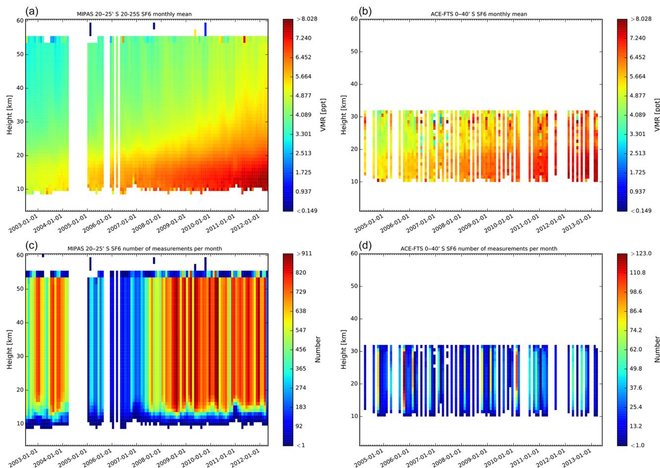
**Figure 7.** SF<sub>6</sub> monthly means of volume mixing ratios profiles (a, b) and the number of measurements in each month (c, d) for MIPAS in the latitude band between 20 and 25° S (a, c) and ACE-FTS in the latitude band between 0 and 40° S (b, d).
