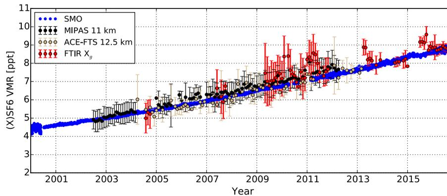
**Figure 5.** Time series of SMO in situ SF<sub>6</sub> daily median (blue), MIPAS SF<sub>6</sub> monthly mean (20–25° S) at 11 km (black), ACE-FTS SF<sub>6</sub> monthly mean (0–40° S) at 12.5 km and FTIR  $X_{\text{SF}_6}$  monthly mean at St Denis and Maïdo (red). For MIPAS, ACE-FTS and ground-based FTIR measurements, the error bar is the standard deviation within 1 month.
