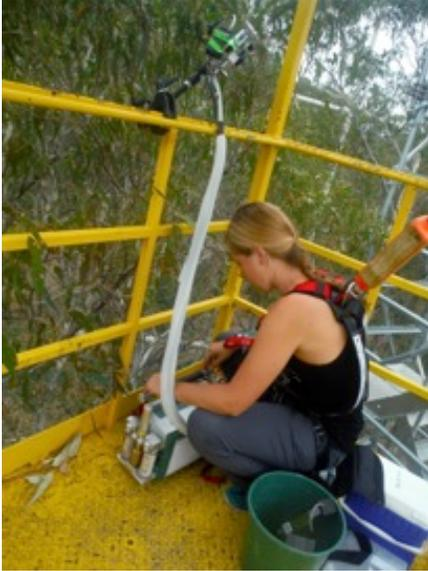
**Figure 6.** Photographic image of Kayla Carey in EucFACE site crane. Leaves from the upper story canopy in the ring were accessed by crane and placed into the leaf chamber of a Li-Cor 6400. The computer system was used to set the specific parameters for the rings and measure the rate physiological processes in the undamaged leaf.
