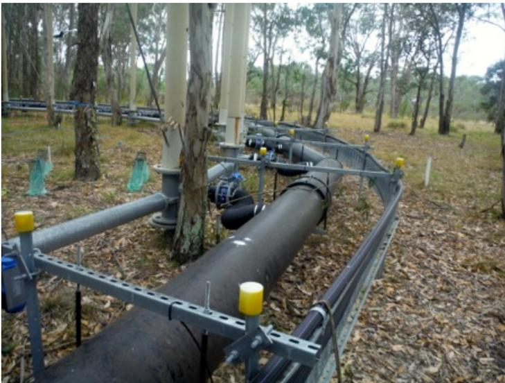
**Figure 5.** Photographic image of the piping system in the EucFACE site. Liquid CO<sub>2</sub> was released by a controlled computer system through interconnected vaporizer pipes that ran through the forest. All piping was elevated from the forest floor to prevent interference with the flow of the ecosystem.
