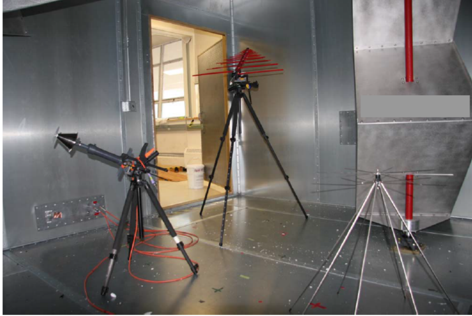
Figure 6.1: The LP antenna inside the large NIST RC, along with the wire discone reference antenna, and one other discone type antenna.
