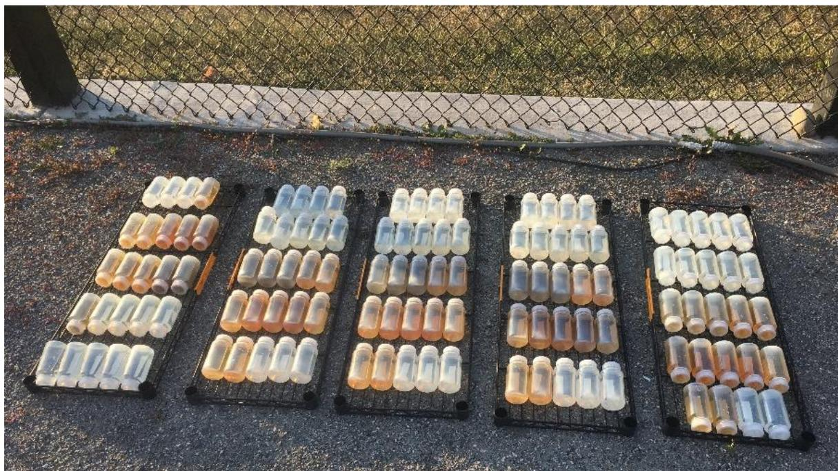
**Figure 5:** Light-exposed leachates were placed on wire racks within the Skywatch Observatory. Samples were opened and turned daily. The leachates were placed in the same order on each rack in triplicate groups. The left most rack, starting from top to bottom and left to right, the leachates appear as: solution blank, 200°C, unburned, 300°C, outside, 400, 550, and 700°C.
