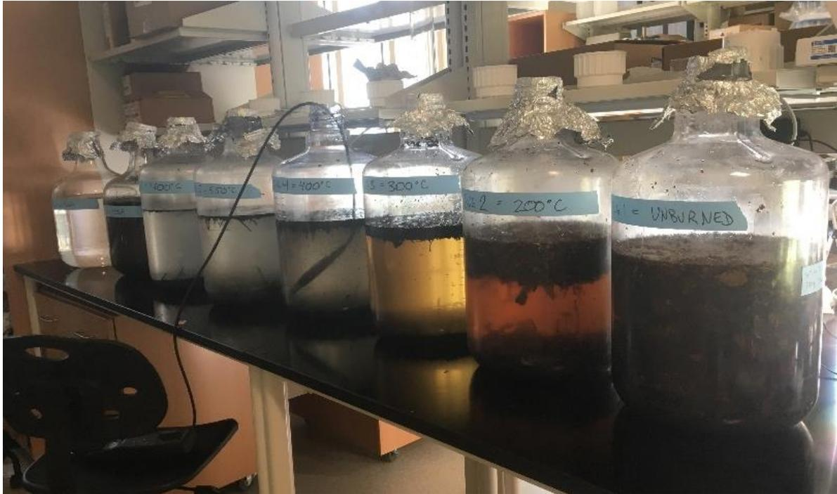
**Figure 4:** Batch leaching of the separate burn treatments. From left to right: solution blank, outside burn, 700, 550, 400, 300, 200°C, and unburned. The burned OM is leaching in a solution of sodium bicarbonate and formaldehyde.
