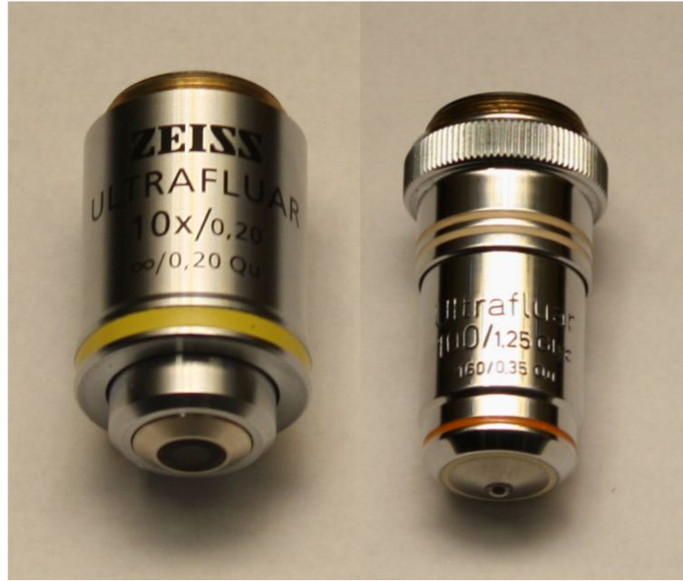
Figure 4.8: Zeiss Ultrafluar objective lenses, corrected in UV and visible bands.
