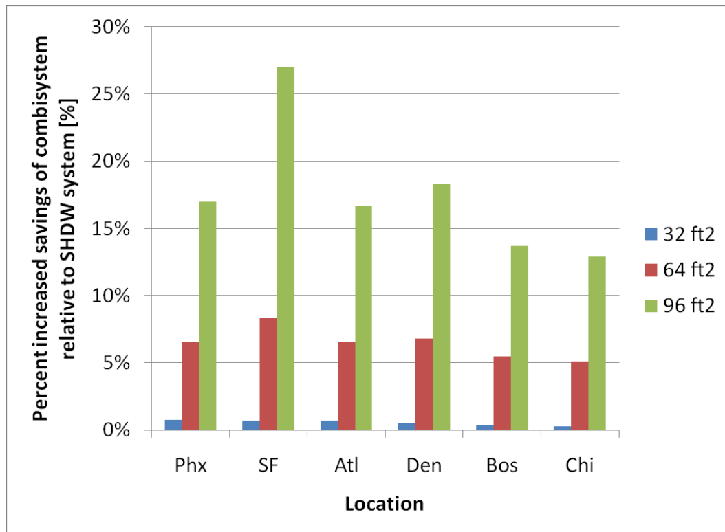
Figure 5.34: Impact of climate on the relative savings increase of the combisystem relative to the SWH for three collector area sizes (Benchmark House/60 gallon draw)
