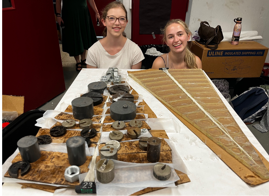
Figure 8: Two completed scintillator tiles for the sEPD. The epoxy is still drying on the tile to the left, so the weights are holding the WSFs in the channels. The epoxy has dried completely on the tile to the right, so it is possible to see the channels where the fibers have been placed.
