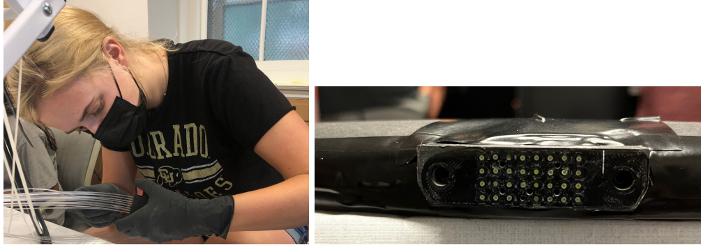
Figure 10: These images show the process of putting the optical fibers through to the connector and polishing them.
