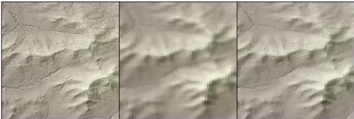
Figure 1.3: Examples of spatial resolution in a DEM. The right panel combines the two spatial resolutions to make a more appropriate display (discussed in section 1.3.1).
